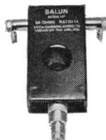
**Decca-KW Balun Mk. II.** The Decca-KW Balun is broadband—3 to 30 MHz, rated up to 2kV p.e.p. 1:1 Ratio 50 ohms "unbalanced" feed to "balanced" output. Waterproof moulded case. Suitable for dipole and Beam aeriels.
