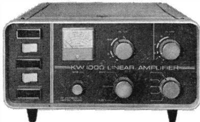
**Decca KW 1000 Linear Amplifier** for SSB and CW 10-80 metres, 1200 watts p.e.p. input SSB, can be "driven" by most 100 watt Transceivers and Transmitters. Employs a pair of T160L Tubes in grounded grid. Pi-section input and output circuits. Built-in 2-4Kv P.S.U.
