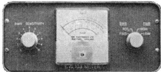
line feeding an Aerial System or Dummy Load (1) Standing Wave Ratio. (2) RF Power with two ranges 0-100 & 0-1000W when used with a 50 ohm Dummy Load.
