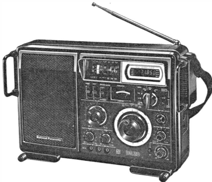
The new Model RF-2800 portable receiver from National Panasonic is "designed specifically for the radio amateur or DX enthusiast." Covering FM/MW/LW and SW from 3.9 MHz, the RF-2800 features an LED 5-digit readout, 2-speed tuning knob with band-spread dial, wide/narrow band selector switch, RF input gain control, variable BFO, external aerial connectors and mains/battery operation. Further information is obtainable from National Panasonic (UK) Ltd., Whitley Road, Slough, Berks.
