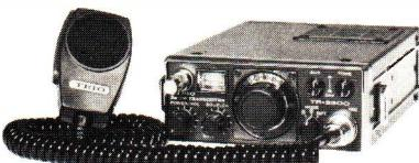
The TR2300 is a remarkable package which combines all the advantages of a portable station with those of a sophisticated mobile set. With the TR2300, you get full band coverage from 144-146 MHz in fully synthesised 25 kHz channels together with 600 kHz repeater shift (and reverse repeater if required) with automatic 1750 Hz tone burst.
