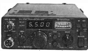
The new TR-7600 is a high performance 2m FM Transceiver with memory, designed to permit multi-channel (400 channel) operation. Featuring the ability of repeater operation. This transceiver brings you all the convenience and versatility in both mobile and fixed station operation.
