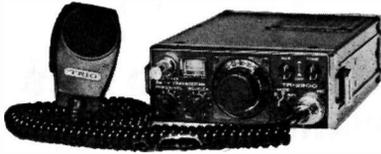
The TR2300 is a remarkable package which combines all the advantages of a portable station with those of a sophisticated mobile set. With the TR2300, you get full band coverage from 144-146 MHz in fully synthesized 25 kHz channels together with 600 kHz repeater shift (and reverse repeater if required) with automatic 1750 Hz tone burst.
