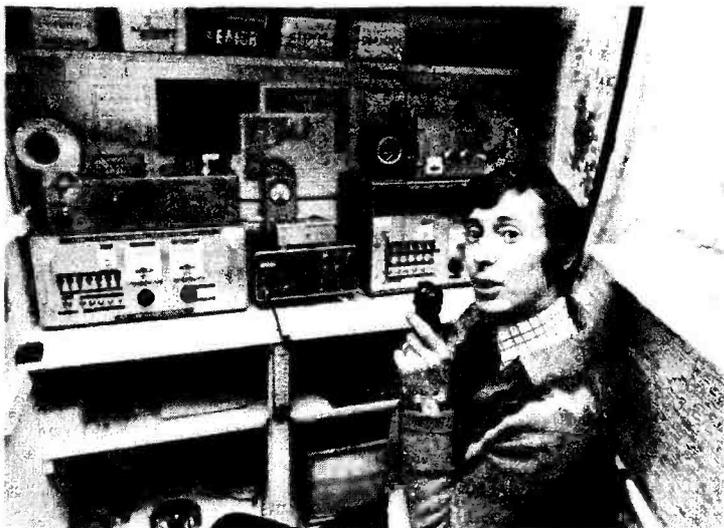
The station of well-known VHF operator Geoff Brown, GJ4ICD, from St. Saviour, Jersey. Left to right: 2 x 4CX250B 2m. amplifier and power supply. Trio TS-700 (since replaced by a TS-770) with a Bird Type 43 power meter above, and a K2R1W 70cm. amplifier with PSU.
