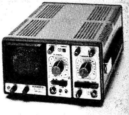
Marketed in the UK by Electronic Brokers Ltd., the West German Hameg HM-307 oscilloscope is aimed specifically at the advanced radio amateur. This 10 MHz, single-trace, 'scope features a sweep circuit using a special LPS trigger technique and built-in component tester, plus several optional accessories. The HM-307 weighs 3.7 kg, and costs £149 plus VAT and carriage. Detailed specifications are available from the marketing firm, at 49/53 Pancras Road, London NW1 2QB. (Tel: 01-837 7781).
