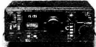
The receiver that revolutionised short wave listening. Full 30 band coverage 200kHz to 30MHz SSB/CW/AM. Both digital and analogue readouts are provided together with 230V or 12V dc operation facilities. Trio engineering at its best and at a very competitive price.
