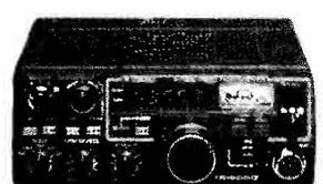
An all mode 2metre transceiver that serves the dual role of mobile and base station. Features include digital readout, 12½ or 25kHz steps in FM, five memories band scanning and a lot more! Send for coloured leaflet.
