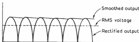
Fig. 2. Smoothed output from a rectifier circuit
