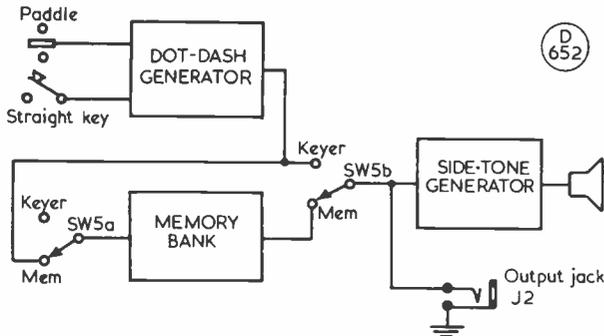
Fig. 9 BLOCK DIAGRAM OF COMBINATION KEYS
