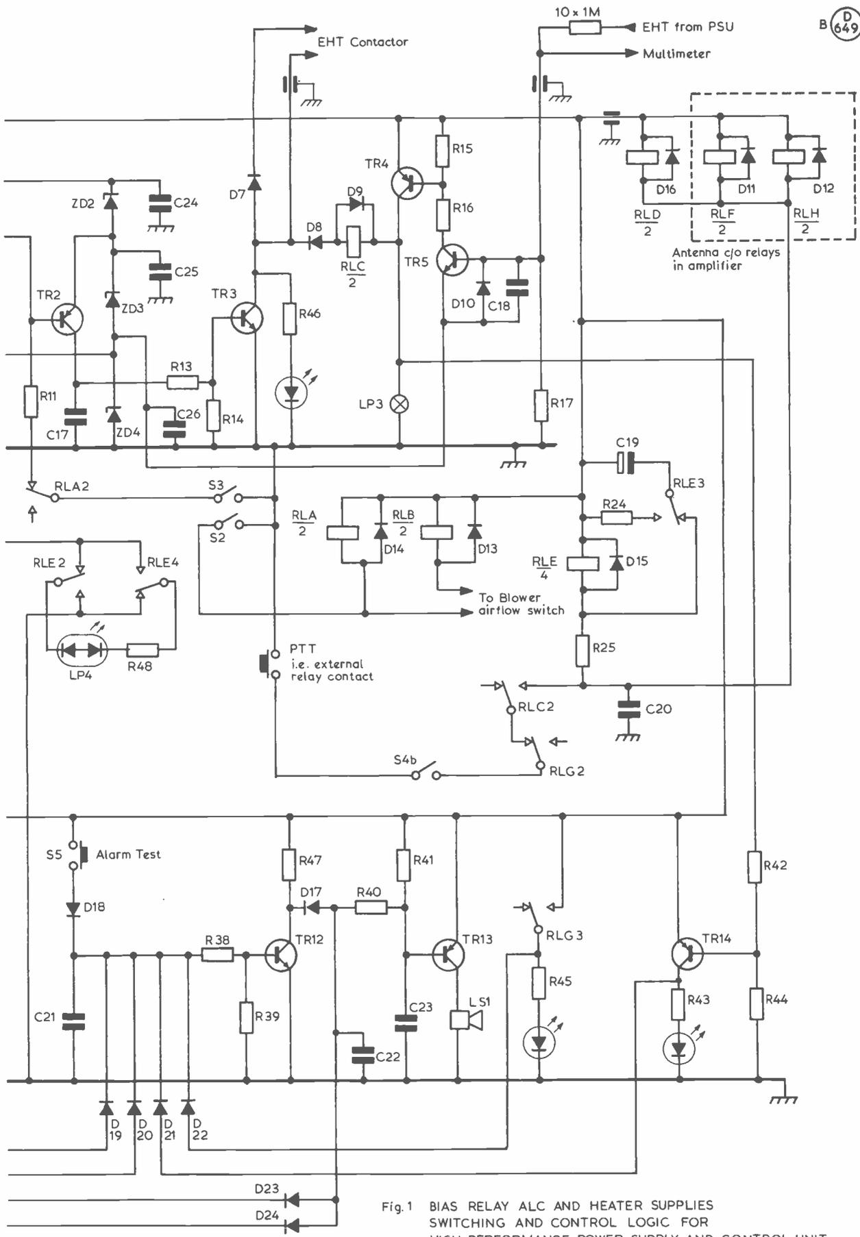
Fig. 1 BIAS RELAY ALC AND HEATER SUPPLIES SWITCHING AND CONTROL LOGIC FOR HIGH PERFORMANCE POWER SUPPLY AND CONTROL UNIT
