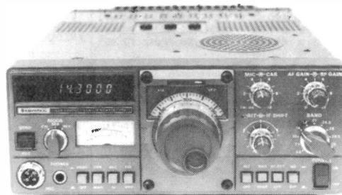
The TS-130S series is an incredibly compact, full-featured, all solid-state HF SSB/CW transceiver for both mobile and fixed operation. It covers 3.5 to 29.7MHz (including the three new amateur bands!) and is loaded with optimum operating features such as digital display, IF shift, speech processor, narrow/wide filter selection (for both SSB and CW modes), and optional (DFC-230) digital frequency controller.
