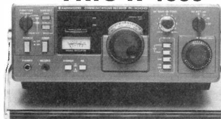
One of the best on the general coverage scene. Full coverage 200kHz to 30MHz with digital frequency readout and clock/timer. Switched selectivity for optimum performance and other features making it a joy to use and first class value for money.
