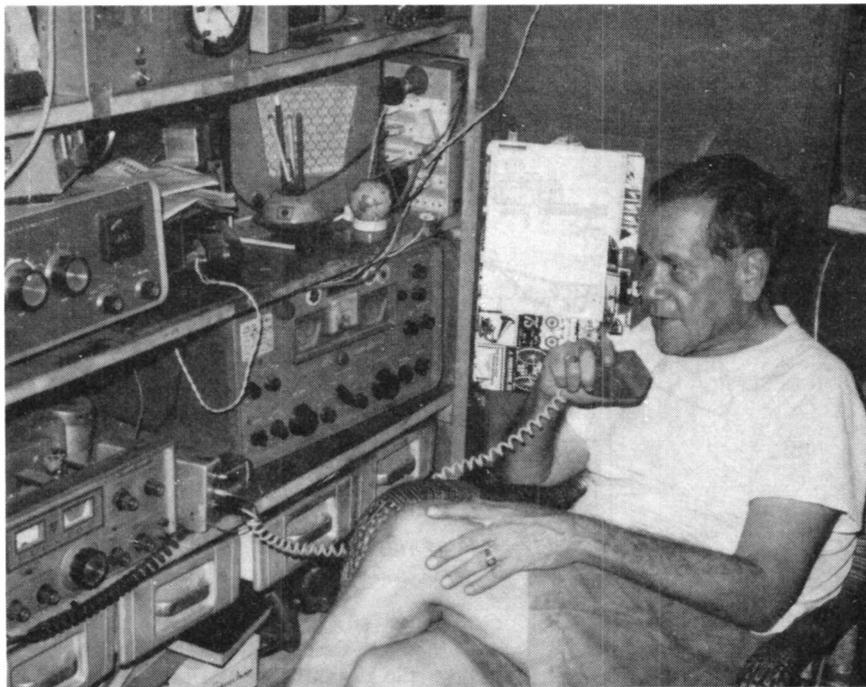
Derek Jeffries, VU2BEJ, is on the air regularly from his QTH in Bombay, and always pleased to QSO UK stations. The rig is an FL-DX400 Tx, HQ-180 Rx and SB-200 linear; antenna is a two-element 3-band quad on top of a 150-ft. high building. Photo: G3ZXX
