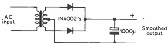
Fig. 1a Full wave rectifier with centre tapped transformer
