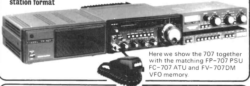
Here we show the 707 together with the matching FP-707 PSU FC-707 ATU and FV-707DM VFO memory.
