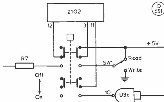
Fig. 8. PUSH BUTTON MEMORY SWITCHING. One circuit is thus required per memory. R7, SW1 and U3c refer to components in Fig. 2, Part 1.
