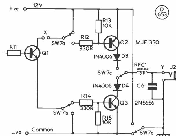
Fig. 10 POSITIVE AND NEGATIVE TRANSISTOR KEYING (SW7 indicated for positive keying.)
