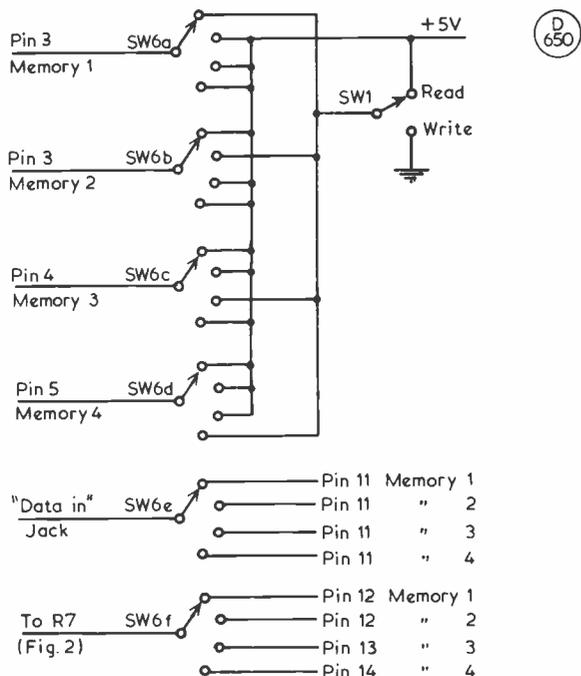
Fig. 7. SWITCH CONNECTIONS USING 6 POLE 4 WAY SWITCH WITH SINGLE 'READ/WRITE' SWITCH.
