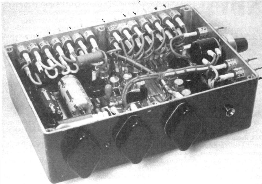
An inside view. The three devices on the side panel are the 78HG relay supply regulator and two 2N3773 transistors for the bias shunt stabiliser and the EHT contactor switch. Adjacent to the latter is its associated LED, whose function is discussed in the text. The wire-wound resistor connected between two feedthroughs in the top left-hand row is R23.
