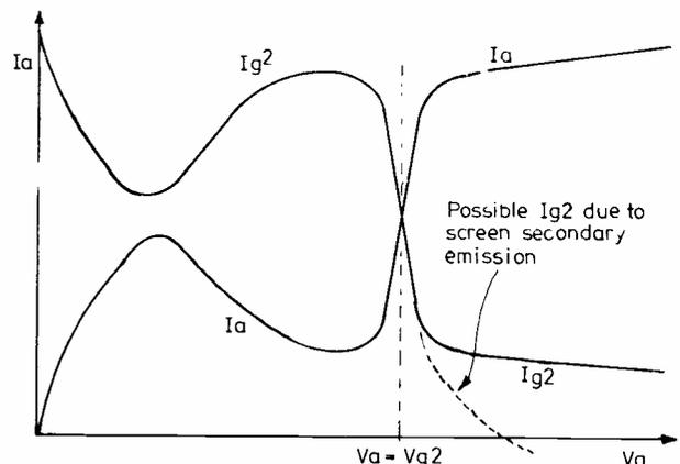
Fig. 2 ANODE AND SCREEN CURRENT CHARACTERISTICS FOR PRACTICAL TETRODE ( $V_{g2}$  CONSTANT)
