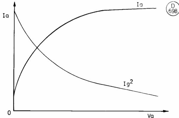
Fig. 1 IDEAL ANODE & SCREEN CURRENT CHARACTERISTICS FOR A TETRODE
