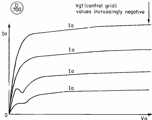
Fig 3 ANODE CURRENT CHARACTERISTICS FOR BEAM TETRODE. (Note 'kink' in Ia at low Va)
