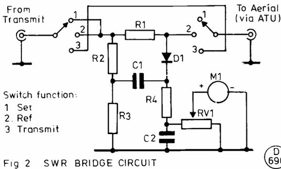
Fig 2 SWR BRIDGE CIRCUIT
