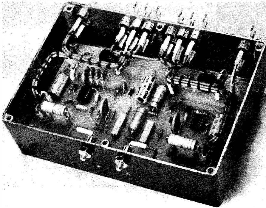
A general view inside the box. The BZY93C75R Zener diodes are bolted directly to the box, with holes for adjustment of the presets directly below them. The 62K/2W resistors are mounted on ceramic stand-offs above the board, and the VDR's across the output of one channel can be seen below the left-hand cableform.
