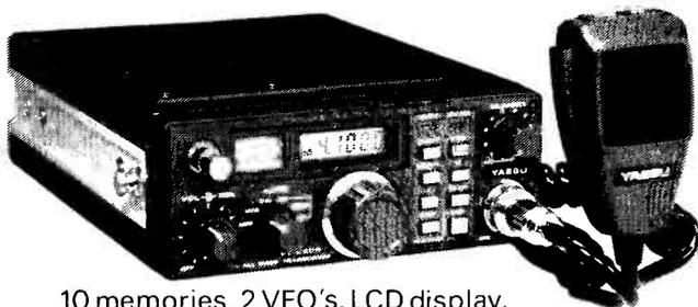
10 memories, 2 VFO's, LCD display, C size battery, easy car mounting tray, 2.5 watts out.
