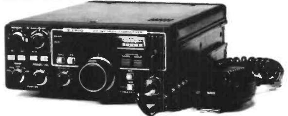
The Trio 9500, a 70 cm multimode mobile giving SSB, FM and CW operation in a compact rig. Add the spacious 70 cm band to your operating.
