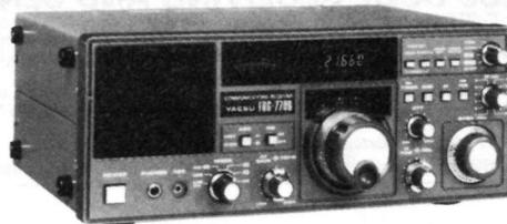
**THE LATEST SOMMERKAMP — FRG 7700 COMMUNICATION RECEIVER.** 150kHz - 30MHz multimode, digital frequency readout, 12 programmable memories, variable bandwidth, built-in clock/timer. P.O.A.
