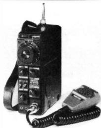
**IC202S/4023W 2M or 70CM SSB PORTABLES.** These Two have been around for a long time and are well proven. SSB, CW and Side-Tone. They come fitted with 144-144.4 (IC202S) and 432-432.4 (IC402). Battery or 12V operation. Built in Antenna or socket for External Antenna.
