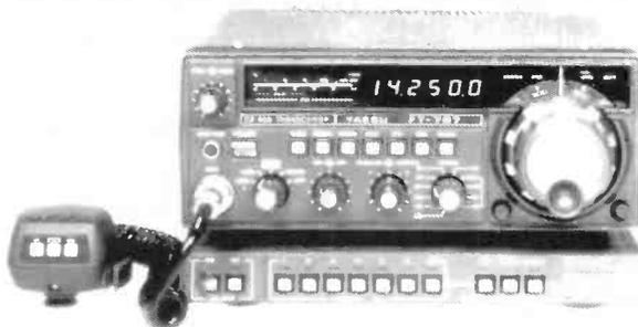
The definitive HF mobile rig, digital, variable IF bandwidth, 100 watts PEP SSB, AM, CW (pictured here with 12 channel memory VFO) Latest bands
