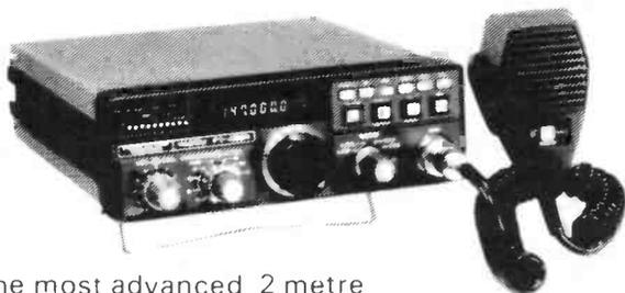
The most advanced 2 metre mobile available today - USB, LSB, FM, CW full scanning with priority channel, 4 memory channel, dual synthesized VFO system.
