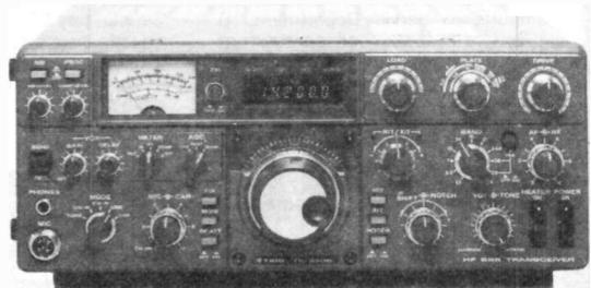
A recent addition to the Trio HF range, and proving amazingly popular is the new TS530S. Designed as a "little brother" to the TS830S, the TS530S uses the same PLL system, same RF boards, same readout system and many other features of the 830 but without the variable bandwidth facility. You do, of course, have the famous Trio I.F. shift system for dodging the QRM.
