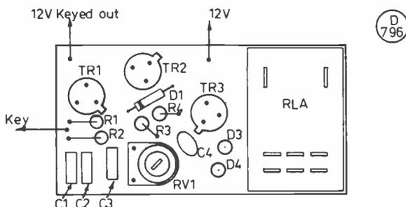
Fig. 6 CHANGEOVER CIRCUIT BOARD (actual size).
