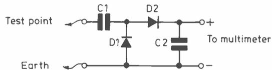
Fig. 8 DIODE RF PROBE
