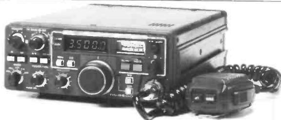
**TR9500** The TR9500, a 70cm multimode mobile giving SSB, FM and CW operation in a compact rig based on the phenomenally successful 2 metre 9000. Combining the convenience of FM with the "DX ability" of SSB on the 70cm band this is the rig all discerning VHF and UHF amateurs have been waiting for.
