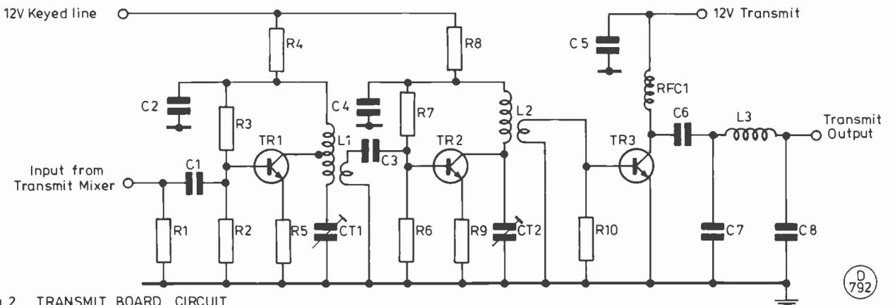
Fig. 2 TRANSMIT BOARD CIRCUIT
