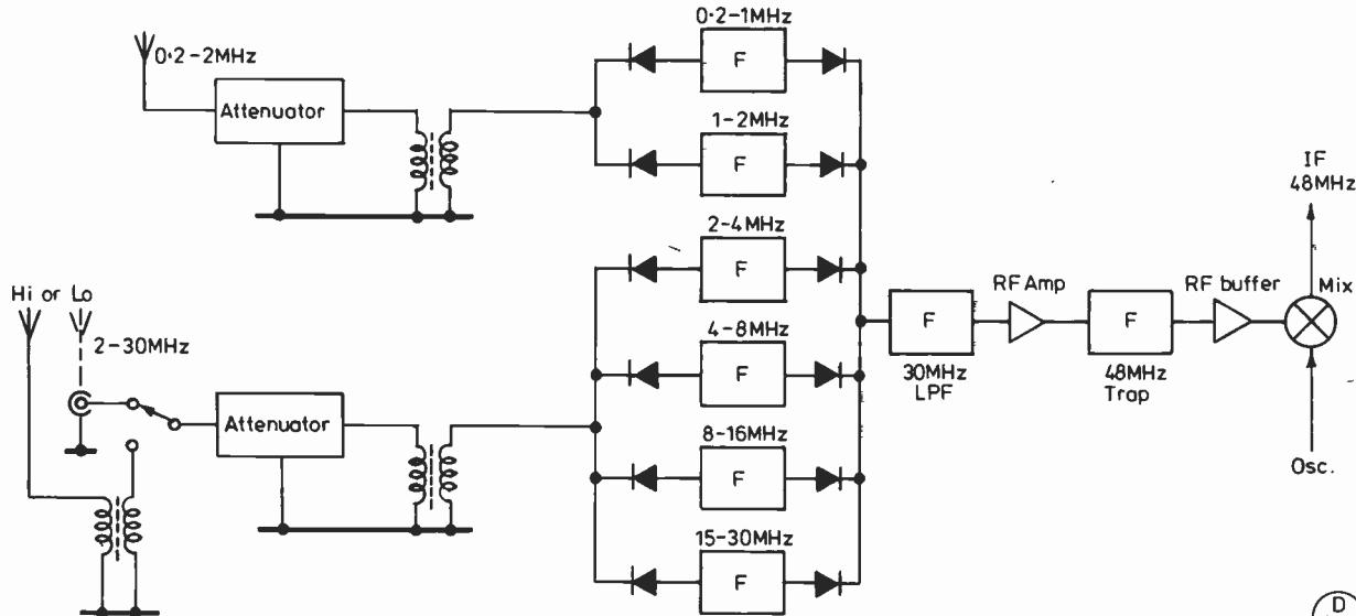
Fig. 7 Signal input circuit layout of R-1000
