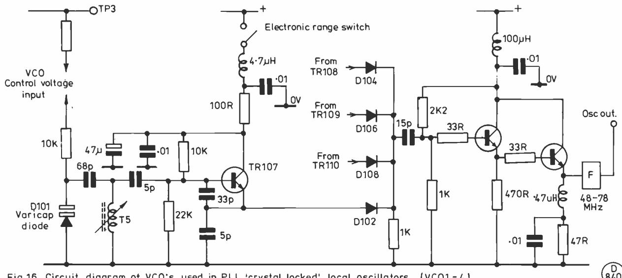
Fig.16 Circuit diagram of VCO's used in PLL 'crystal locked' local oscillators (VCO1-4)
