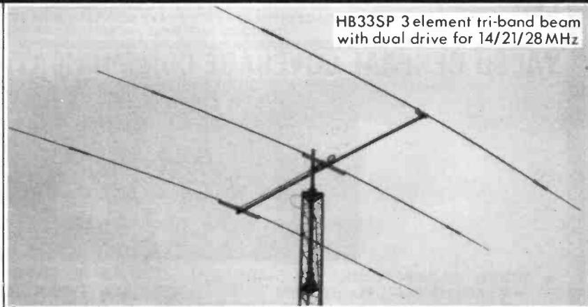
HB33SP 3 element tri-band beam with dual drive for 14/21/28 MHz
