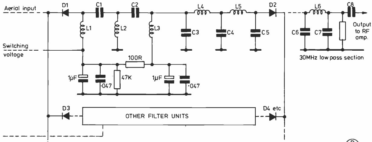
Fig. 8 RF Input bandpass filters
