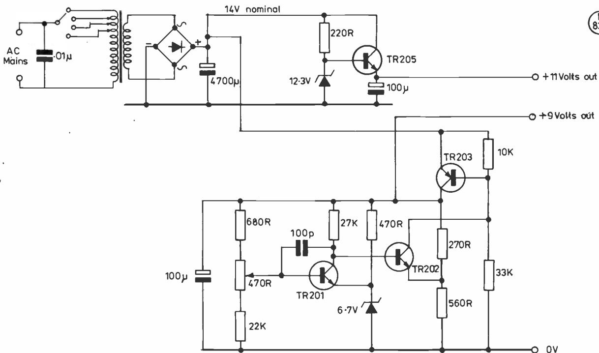
Fig.14 Mains Power Circuit for the R-1000
