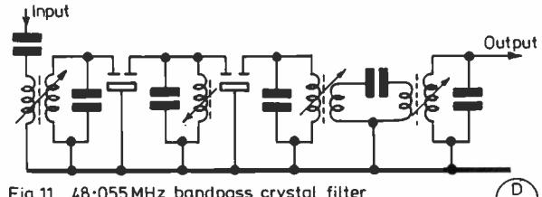
Fig.11 48.055 MHz bandpass crystal filter
