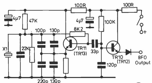
Fig.13 Crystal BFO oscillator circuit used in USB/LSB carrier injection
