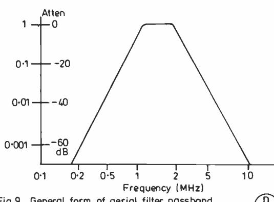
Fig. 9 General form of aerial filter passband (1-2 MHz filter illustrated).
