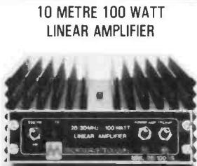
This all new 10 metre solid-state linear amplifier is intended for use with any existing 28MHz equipment having an output power of up to 10 watts. When used with such a drive source this unit will provide an output power of 100 watts on SSB and FM and 40 watts on AM. The linear amplifier and the ultra low noise receive preamp can both be independently switched in and out of circuit, due to the inclusion of sophisticated switching circuitry controlled by front panel mounted switches.
