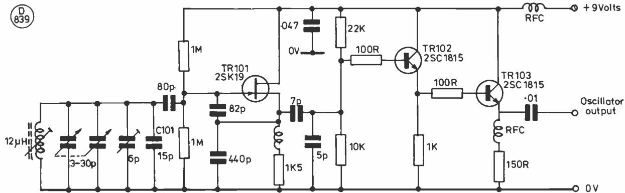
Fig.15 The Variable Frequency Oscillator
