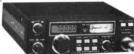
**2m, 25W, FM, £ 239 inc. FT230R** 6" x 2" x 7", 12½/25kHz, ±600kHz, special LCD display, 10 memories, memory and band scan, RX priority feature, two independent VFO's.
