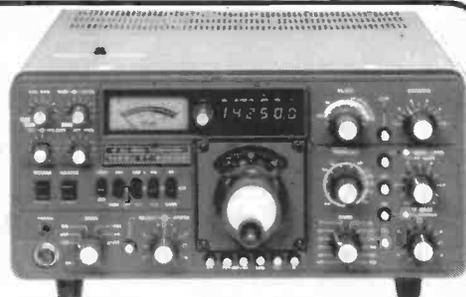
The YAESU world famous pace-setter with the acknowledged unbeatable reputation 160 thru 10 metres including the new WARC bands. All-mode capability, SSB, CW, AM, FSK and FM transmit and receive. Teamed with the FTV-901R transverter coverage extends to 144 & 430MHz.
