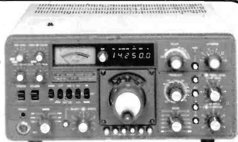
The YAESU world famous pace-setter with the acknowledged unbeatable reputation. 160 thru 10 metres including the new WARC bands. All-mode capability, SSB, CW, AM, FSK and FM transmit and receive. Teamed with the FTV-901R transverter coverage extends to 144 & 430MHz.
