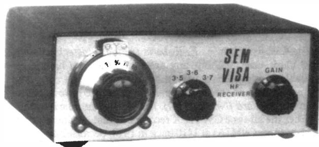
S.E.M. announce the availability of the 'Visa', their new receiver for the amateur. Priced at £39.00, it is intended as a receiver for the beginner or as an additional shack Rx. Measuring only 2½ x 6 x 3 inches, coverage is 3.5 to 3.8 MHz (80 metres in three 100 kHz bands), audio output 2 watts, selectivity ±2 kHz, and sensitivity 1 μV. Full specifications are obtainable from S.E.M., Union Mills, Isle of Man.
