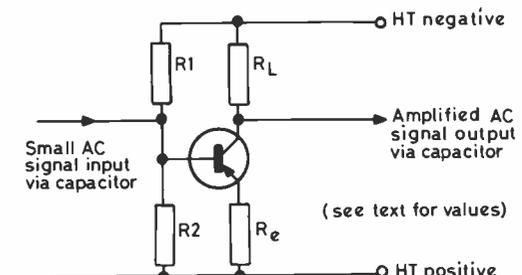
(c) DC conditions around a PNP germanium transistor
