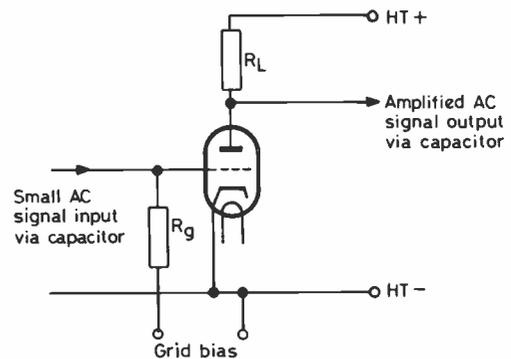
(a) DC conditions on the electrodes of a triode valve.
