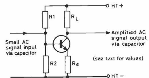
(b) DC conditions around an NPN silicon transistor
