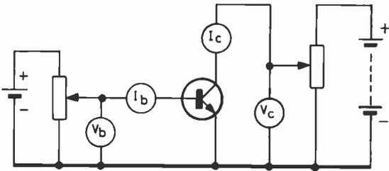
(b) SILICON NPN TRANSISTOR - See Fig.6 for text and discussion. For PNP transistor, reverse polarity of both batteries.
