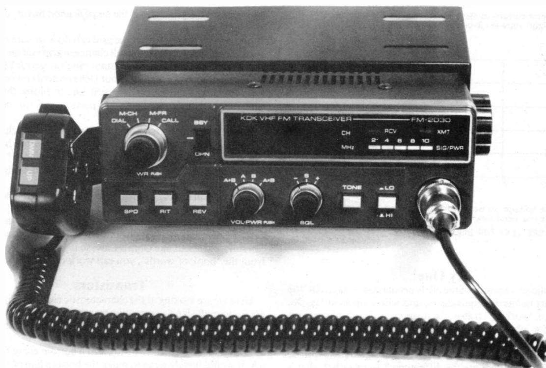
Fig. 1. Front view of the KDK FM-2030, two metres FM transceiver. The detachable mobile mounting bracket is supplied with the set, is adjustable for tilt angle and can be fitted either to the top or bottom. The microphone clip can be fitted either side and the 500 ohms dynamic microphone supplied has "Up" and "Down" buttons for remote channel switching.
