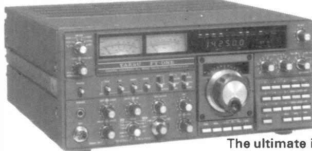
The ultimate in HF transceivers - the superb FT-ONE provides continuous RX coverage of 150KHz-30MHz plus all nine amateur bands (160 thru 10m). All-mode operation LSB, USB, CW, FSK, AM, \*FM • 10 VFO system • FULL break-in on CW • audio peak filter • notch filter • variable bandwidth and IF shift • keyboard scanning and entry • RX dynamic range over 95dB! and NO band switch!!!
