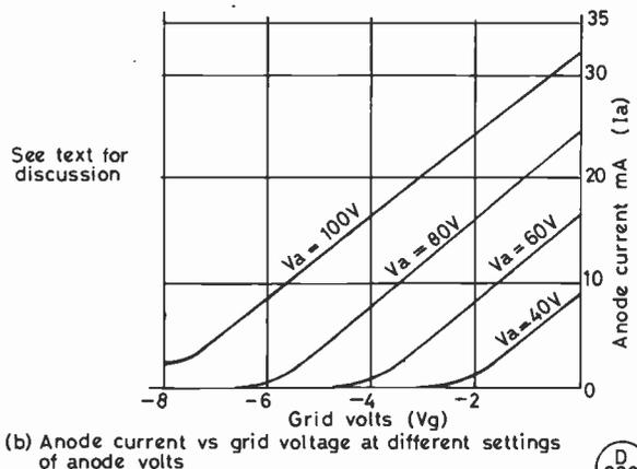
(b) Anode current vs grid voltage at different settings of anode volts
