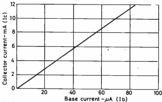
(b) Collector current vs Base current for fixed value of collector voltage (3volts). Note the linearity
