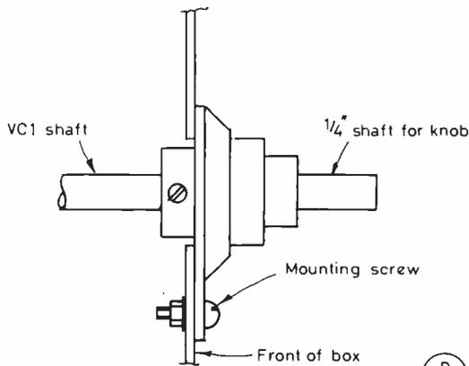
Fig 6 VERNIER DRIVE MOUNTING
