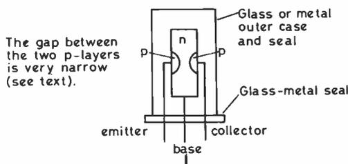
Fig.1 BASIC CONCEPT OF GERMANIUM JUNCTION TRANSISTOR
