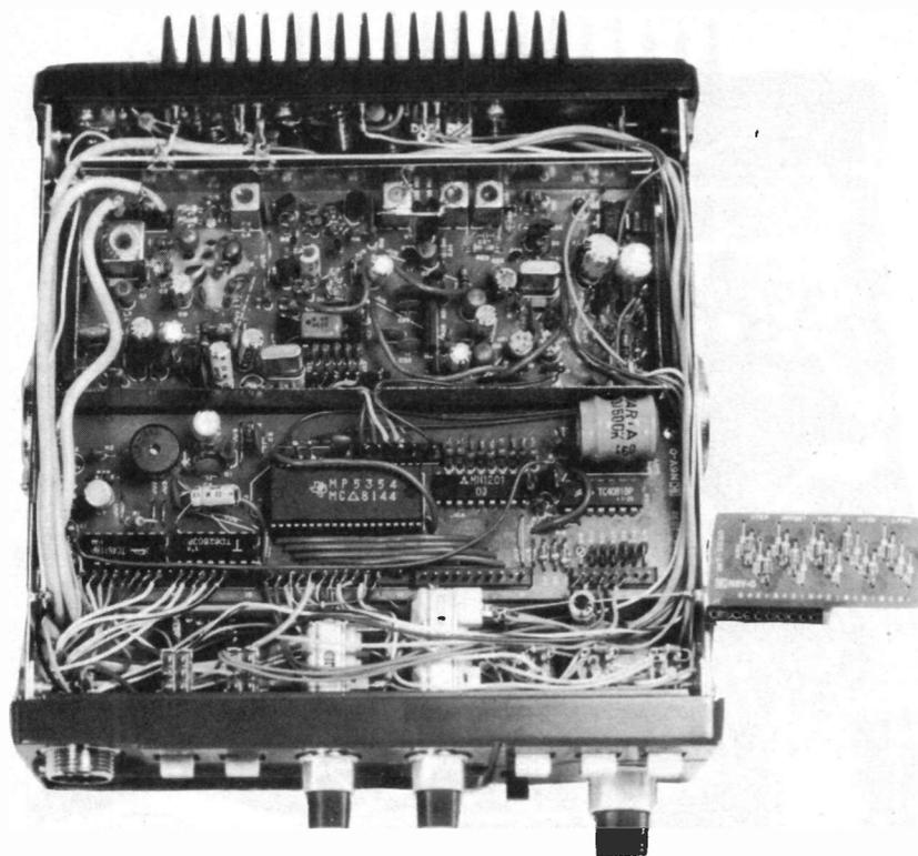
Fig. 3. Bottom view. The board behind the front panel is the Control Unit with the CPU chip in the middle. The "loose" board at the right plugs into the 9-pin socket at the bottom right of the CPU and is the Initialize Unit containing the diode matrices for programming the CPU. The memory back-up battery is in the top right corner of this board. The rear p.c.b. accommodates the phase locked loop circuitry. Photo by T. Traill
