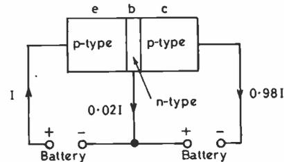
Fig.2 Basic connections to demonstrate transistor action
