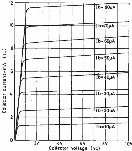
(a)  $I_c/V_c$  curves for typical small signal germanium transistor
