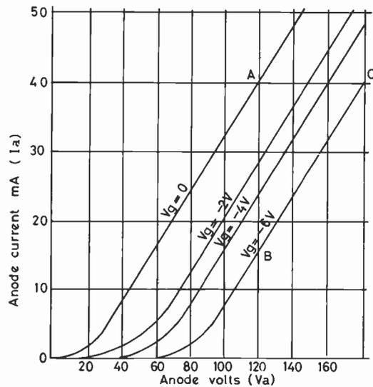
(a) Characteristic curves of a triode at different settings of Vg
