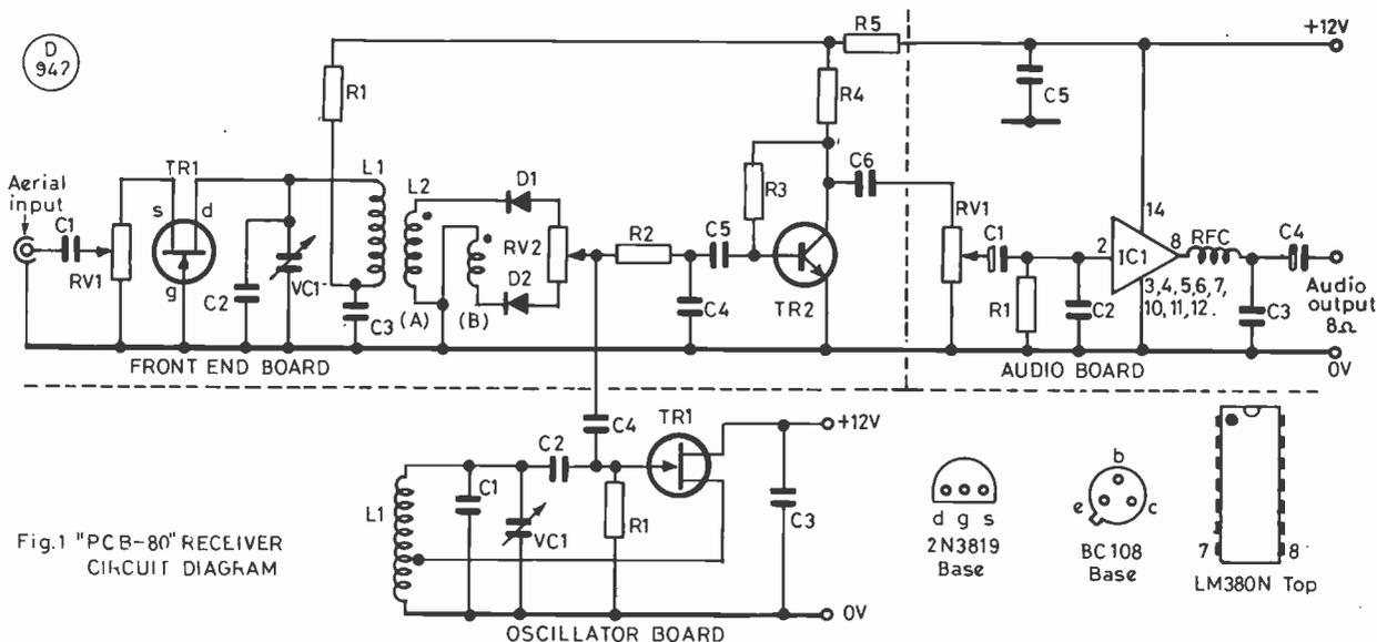
Fig.1 "PCB-80" RECEIVER CIRCUIT DIAGRAM
