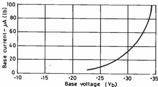
(c) Base voltage vs Base current at fixed value of  $V_c$  (3V) Note the non-linearity.
