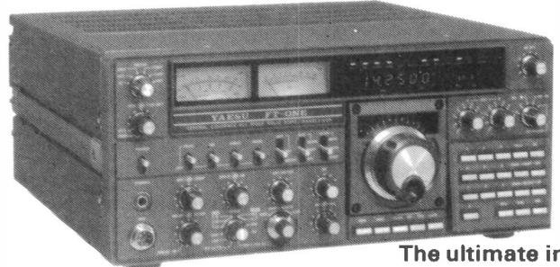
The ultimate in HF transceivers - the superb FT-ONE provides continuous RX coverage of 150KHz-30MHz plus all nine amateur bands (160 thru 10m). All-mode operation LSB, USB, CW, FSK, AM, \*FM • 10 VFO system • FULL break-in on CW • audio peak filter • notch filter • variable bandwidth and IF shift • keyboard scanning and entry • RX dynamic range over 95dB! and NO band switch!!!
