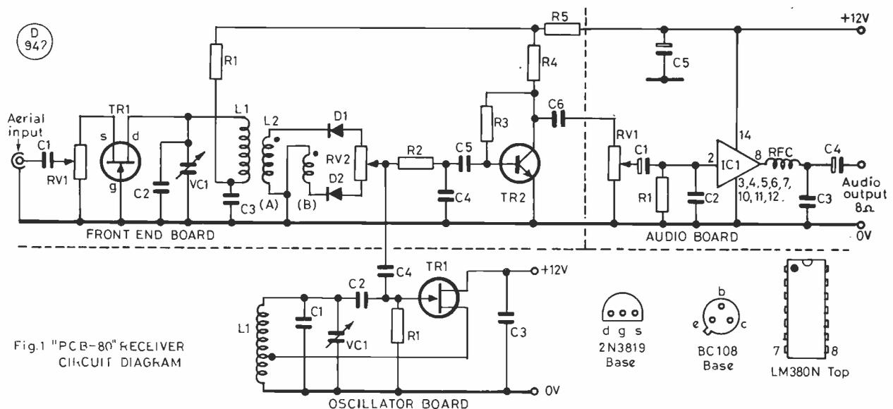
Fig.1 "PCB-80" RECEIVER
