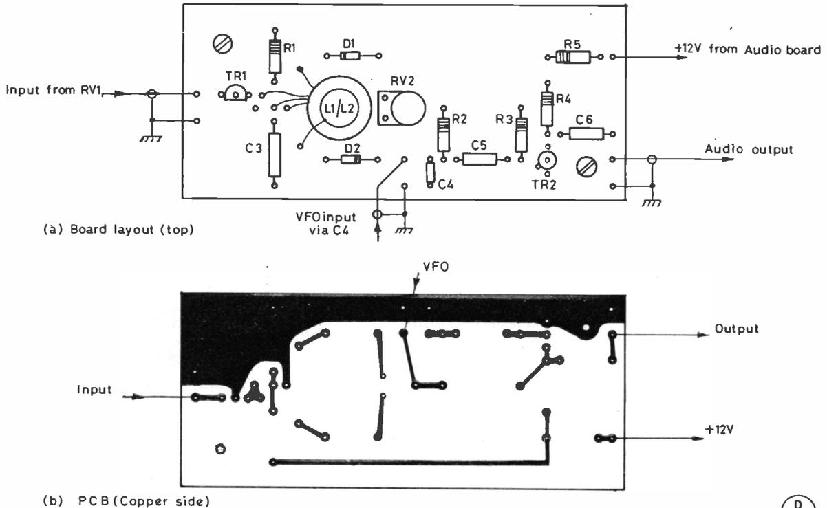
Fig.3 FRONT END BOARD (Actual size)
