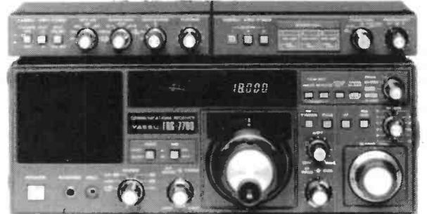
YAESU's top of the range receiver. All-mode capability, USB, LSB, CW, AM and FM 12 memory channels with back-up. Digital quartz clock feature with timer. Pictured here with matching FRT-7700 Antenna tuner and FRV-7700 VHF converter.
