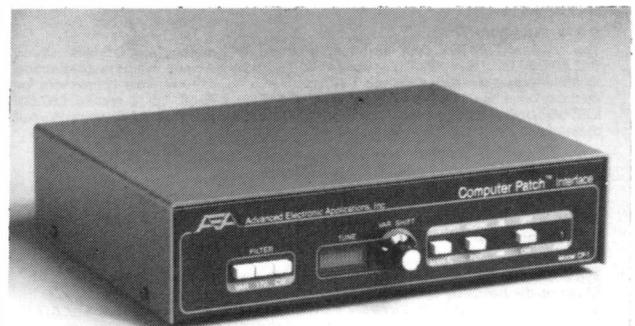
The AEA CP-1 Computer Patch, shown above, converts a transceiver and personal computer into a full function RTTY station. Priced at £169 including VAT and carriage, the CP-1 is available from I.C.S. Electronics Ltd., P.O. Box 2, Arundel, West Sussex BN18 0NX (tel: 024365-590).
