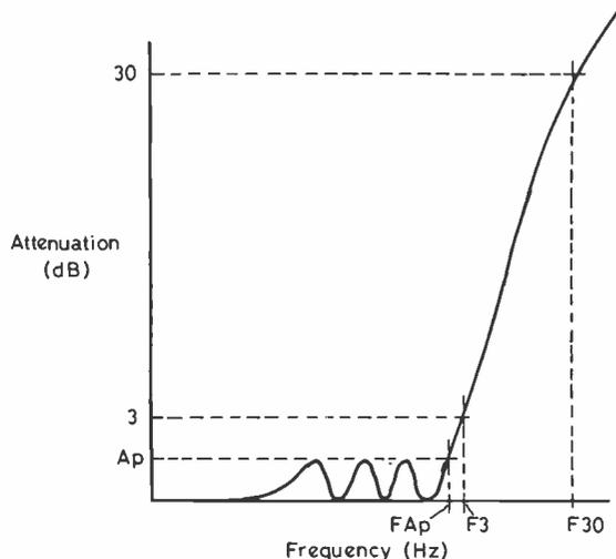
(b) Typical attenuation response. The passband attenuation ripple amplitude (Ap) is exaggerated for clarity.
