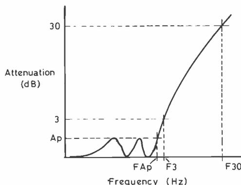
(b) Typical attenuation response. The passband ripple amplitude ( $A_p$ ) is exaggerated for clarity.
