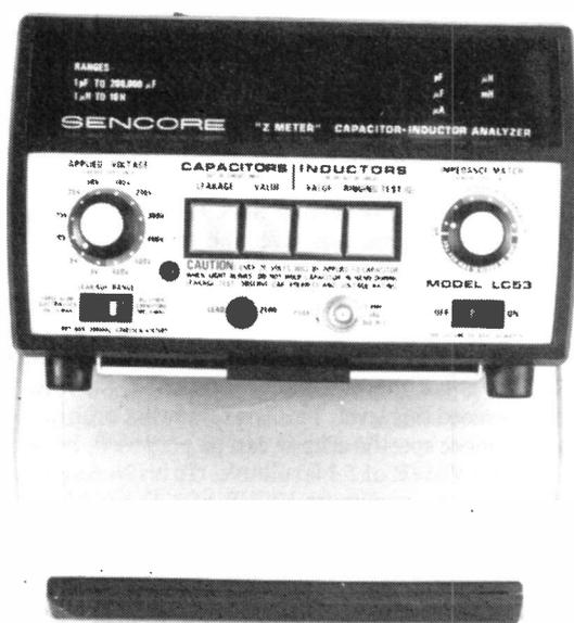
The LC53, shown above, offers dynamic testing for capacitors, coils, SCR's and Triac's. For further details contact Mike Dawson, *Fieldtech Heathrow Ltd.*, Huntavia House, 420 Bath Road, Longford, Middlesex UB7 0LL. Tel. 01-897 6446. Telex 23734.
