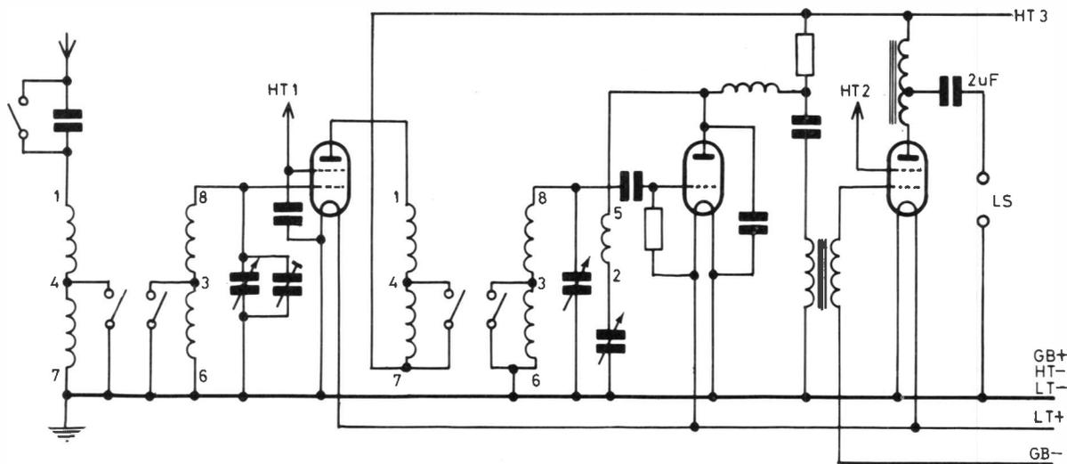
Fig. 1(c) A 3 VALVE CIRCUIT OF THE EARLY THIRTIES. (The "TELSEN JUPITER SG3" Kit)
