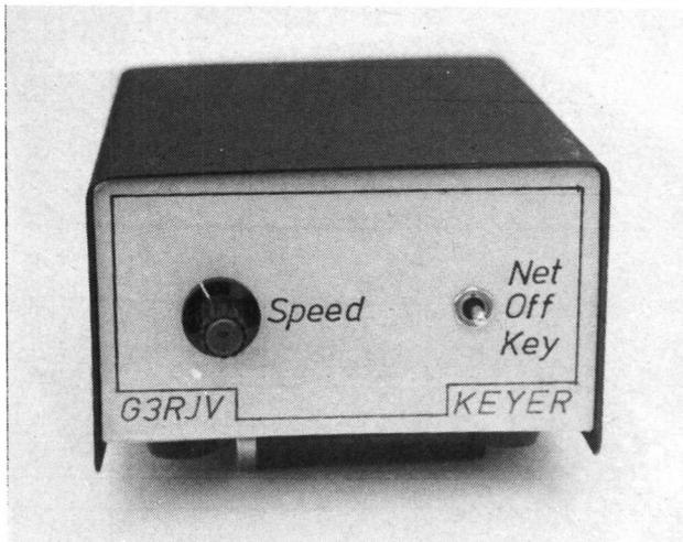
An electronic keyer mounted in a "double U" type case, with a card front panel marked with lettering (Rotring pen and stencil) and finished with plastic film.
