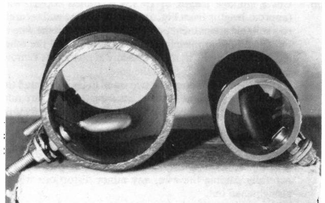
Fig. 7. Discrete component traps; note the capacitors located inside the coil formers.
