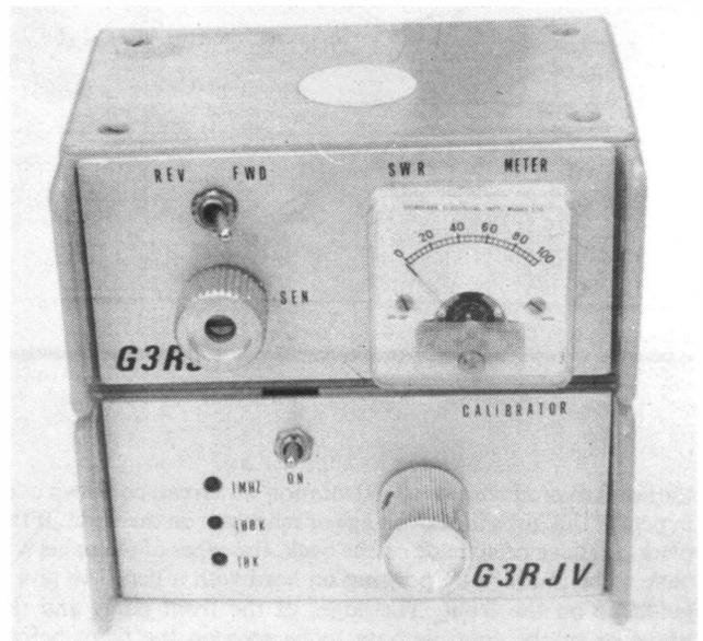
Two front panels in aluminium finish using the technique described in the article. The cases are surplus G.P.O. plastic boxes with added aluminium fronts. The units are the SWR Bridge and Calibration Oscillator described in the *Short Wave Magazine* series "Plug in Your Soldering Iron and Begin Here".
