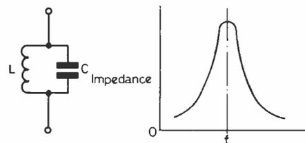
Fig. 1b PARALLEL RESONANT CIRCUIT
