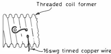
Fig. 6b. COIL CONNECTION DETAIL
