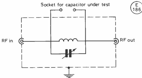
Fig. 3 THE G3XAP CAPACITOR COMPARATOR
