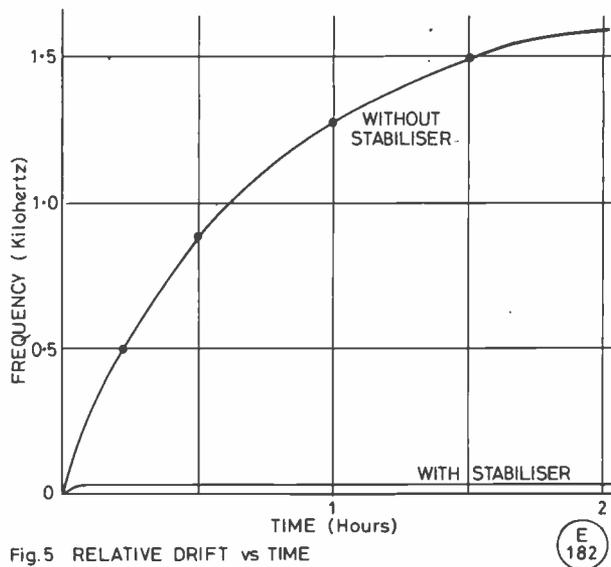
Fig.5 RELATIVE DRIFT vs TIME
