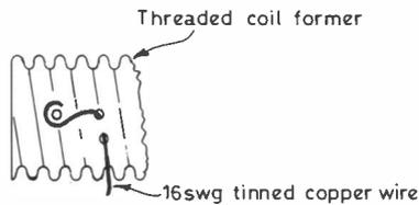
Fig. 6b. COIL CONNECTION DETAIL
