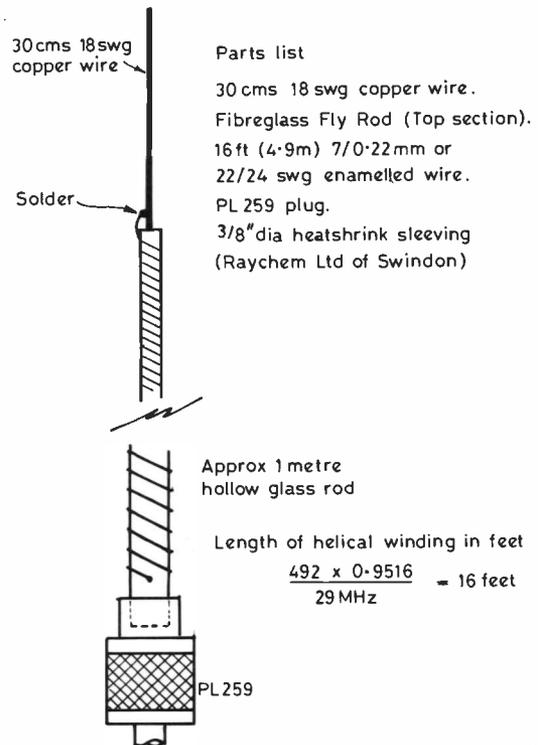
Fig.1 10 METRE HELICAL MOBILE ANTENNA
