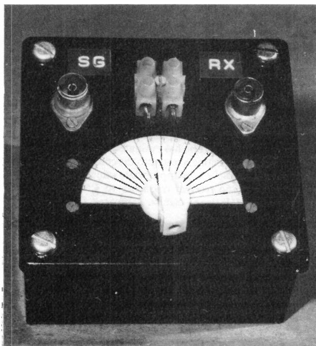
Fig. 2(b). An external view of the G3XAP Capacitor Comparator.
