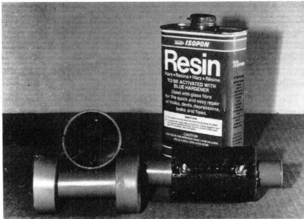
Fig. 8. A partly-assembled mould, plus a fully encapsulated trap.
