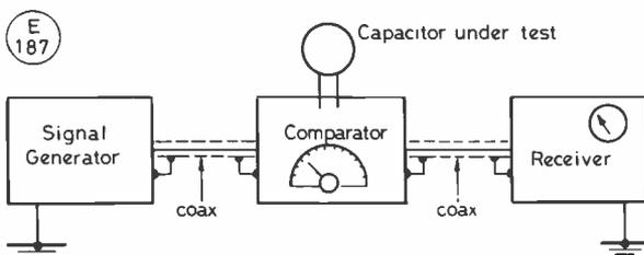
Fig. 4 TEST SET-UP FOR USING THE CAPACITOR COMPARATOR
