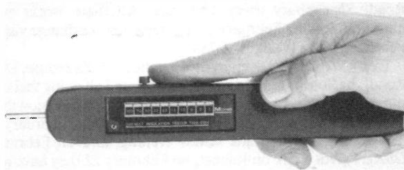
Shown here is the *Osborne Electronics Model 4100*, a new 500-volt, low-cost, hand-held, self-contained insulation tester which, the maker says, offers radical improvements over existing test units. The Model 4100 has many interesting features, and for further information contact the manufacturer, *Osborne Electronics*, Ryde, Isle of Wight. Tel: 0983-63622. Telex: 86363.
