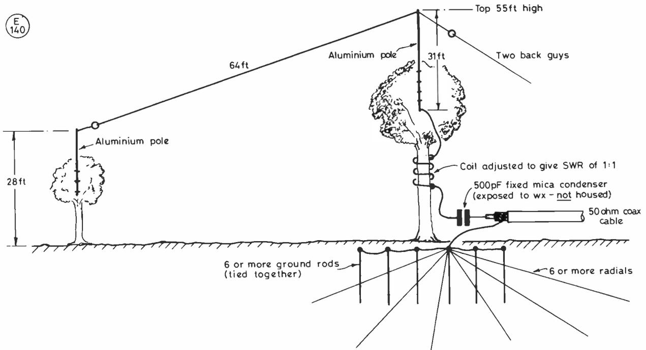
THE W1TX 160m INVERTED "L" TREE ANTENNA
