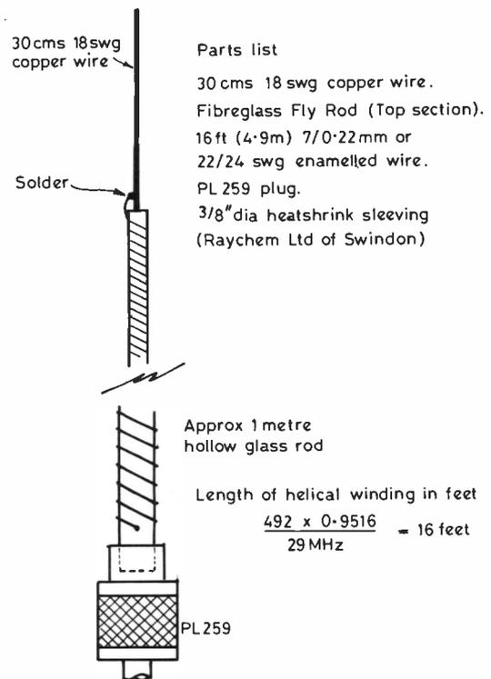
Fig.1 10 METRE HELICAL MOBILE ANTENNA
