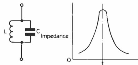
Fig. 1b PARALLEL RESONANT CIRCUIT
