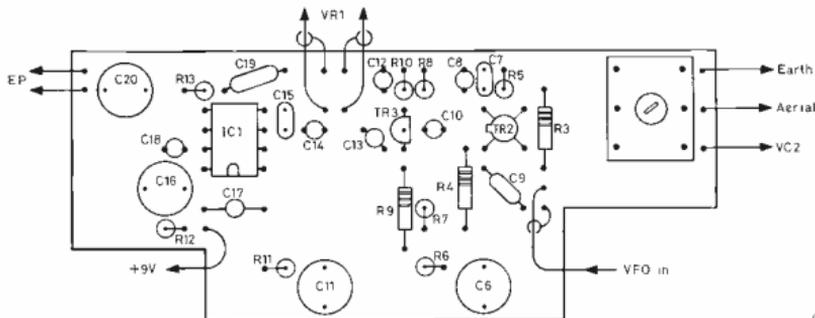
Fig 3 MINI MONITOR MAIN BOARD LAYOUT
