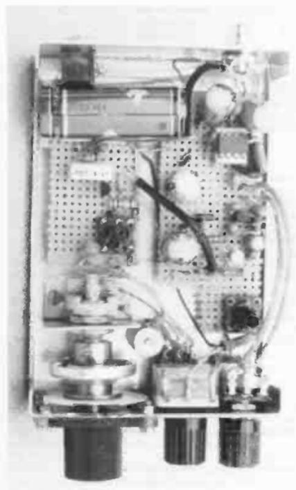
An inside view of the Mini-Monitor receiver, showing the VFO board behind the slow-motion drive assembly, with the main board behind RV1 and VC2. photo: Jo-Anna
