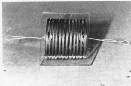
Fig. 2. A discrete component trap — an alternative approach. Note that the coil former consists of a drilled perspex sheet.
