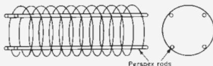
Fig 1 COIL STOCK MANUFACTURED WITH WIRE COILED ONTO PERSPEX RODS
