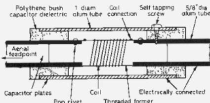
Fig 5 G3VMC'S METHOD OF CONSTRUCTION OF COAXIAL TRAPS
