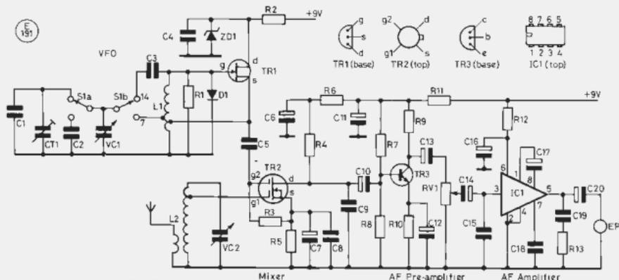
Fig 1 MINI-MONITOR CIRCUIT DIAGRAM
