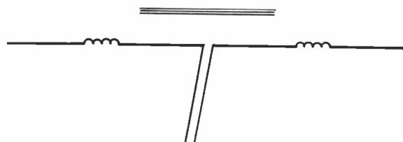
Fig.1c. EQUIVALENT CIRCUIT OF THE TWO-BAND TRAPPED DIPOLE WHEN OPERATED AT FREQUENCY  $f_2$
