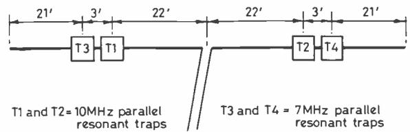
Fig.8 TRI-BAND TRAPPED DIPOLE FOR 3.5/7/10MHz
