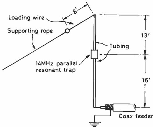
Fig.10 THE "XAP 2V" INVERTED-L FOR 14/21MHz
