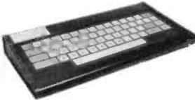
This microprocessor-based product is the ultimate in 'electronic keyers' and will send both live and stored messages in the speed range 12–30 wpm.
