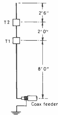
Fig.9 TRAPPED VERTICAL FOR 14/21/28 MHz
