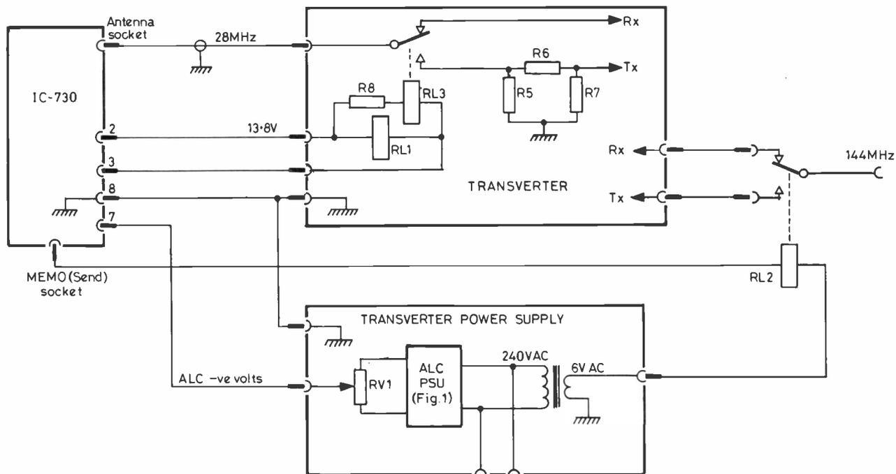
Fig. 2 TRANSCEIVER, TRANSVERTER AND POWER SUPPLY INTERCONNECTIONS
