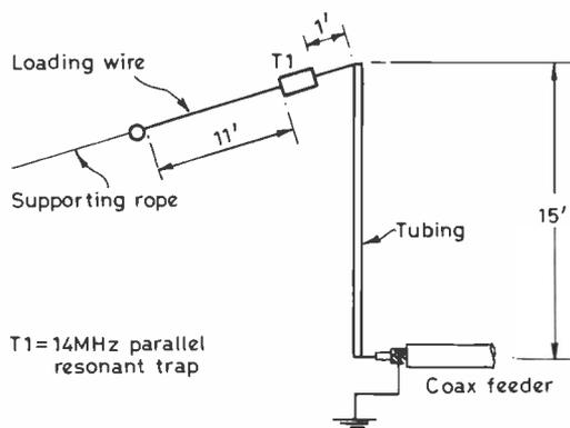
Fig.12 A 4-BAND INVERTED-L
