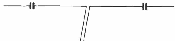
Fig. 3. EQUIVALENT CIRCUIT OF A TWO-BAND TRAPPED DIPOLE WHEN OPERATED ON A FREQUENCY HIGHER THAN THE RESONANT FREQUENCY OF ITS TRAPS.
