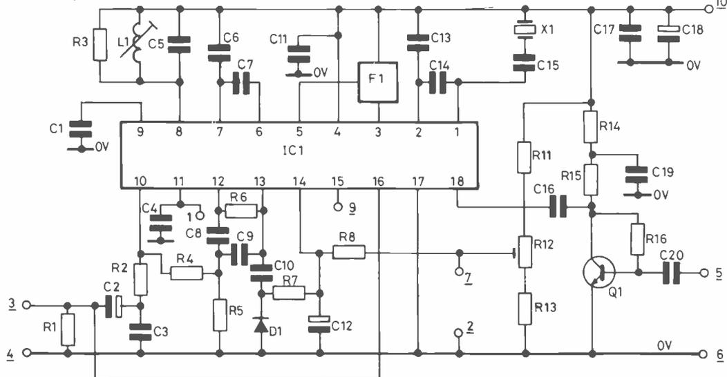
Fig. 2 FM707 DEMODULATOR CIRCUIT
