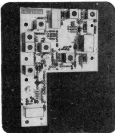
**IC 271 Replacement Front-End — RPCB 271ub**
