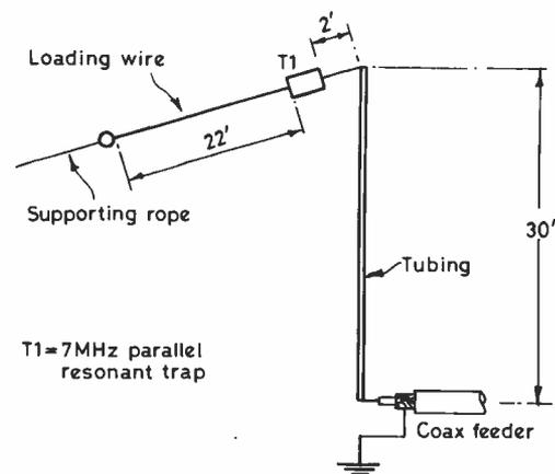
Fig.11 A 5-BAND INVERTED-L
