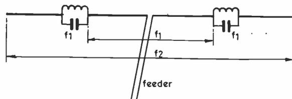
Fig.1a A TWO-BAND TRAPPED DIPOLE
