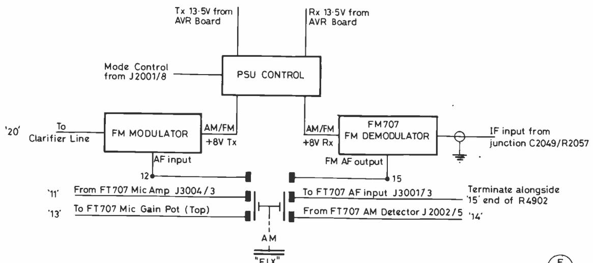
Fig.1 FM CONVERSION FOR FT707 - INTERWIRING DIAGRAM
