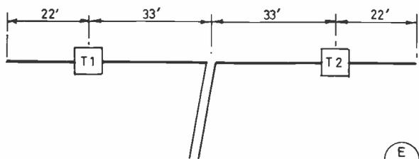
Fig.4 THE W3DZZ MULTI-BAND TRAPPED DIPOLE.
