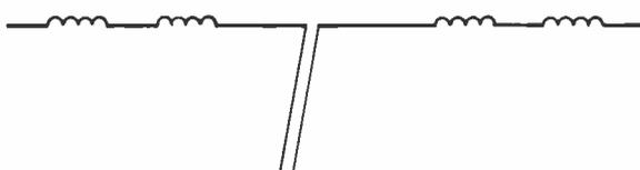
Fig. 2c. EQUIVALENT CIRCUIT OF THE THREE-BAND TRAPPED DIPOLE WHEN OPERATED ON 1.8MHz
