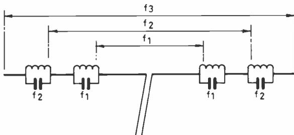
Fig. 2a. A THREE-BAND TRAPPED DIPOLE
