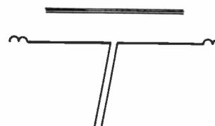
Fig.1b. EQUIVALENT CIRCUIT OF THE TWO-BAND TRAPPED DIPOLE WHEN OPERATED AT FREQUENCY  $f_1$
