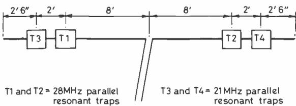
Fig.7 TRI-BAND TRAPPED DIPOLE FOR 14/21/28MHz.
