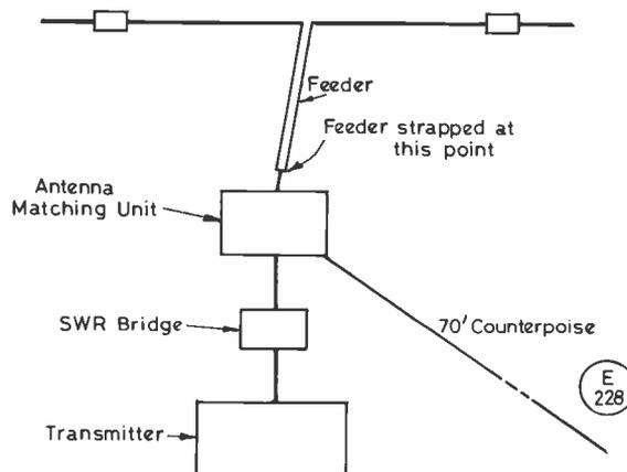
Fig.6 THE 4-BAND TRAPPED DIPOLE OPERATING ON 3.5MHz
