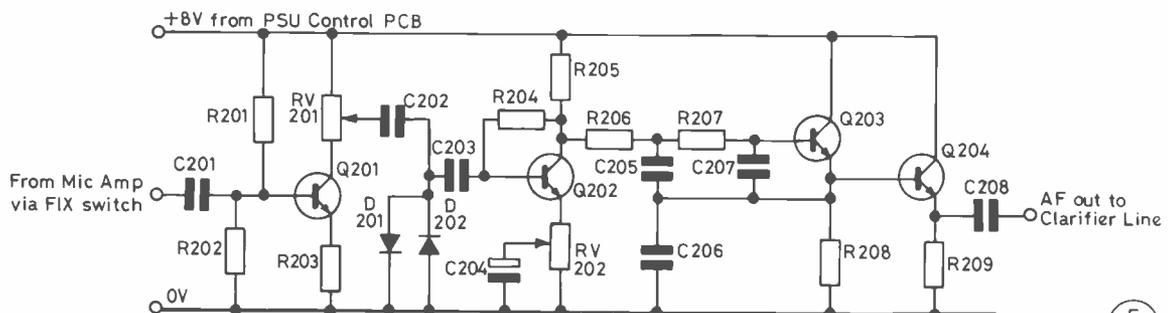
Fig.5 FM CONVERSION FOR FT-707 MODULATOR CIRCUIT
