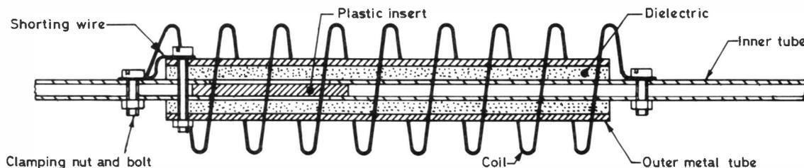
Fig. 7 DIAGRAMMATIC REPRESENTATION OF THE ALTERNATIVE COAXIAL TRAP
