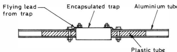
Fig. 6 ENCAPSULATED TRAP SECURED TO ALUMINIUM TUBING.
