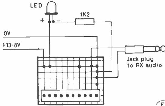
Fig.5 MOTHERBOARD END CONNECTOR -TEST JIG.
