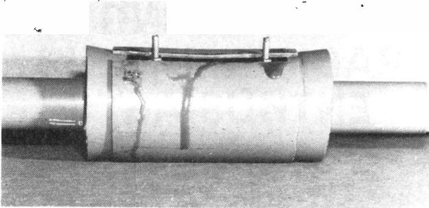
Fig. 3. The assembled mould with a trap in position.
