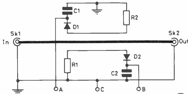
Fig.1 CIRCUIT OF THE SWR BRIDGE
