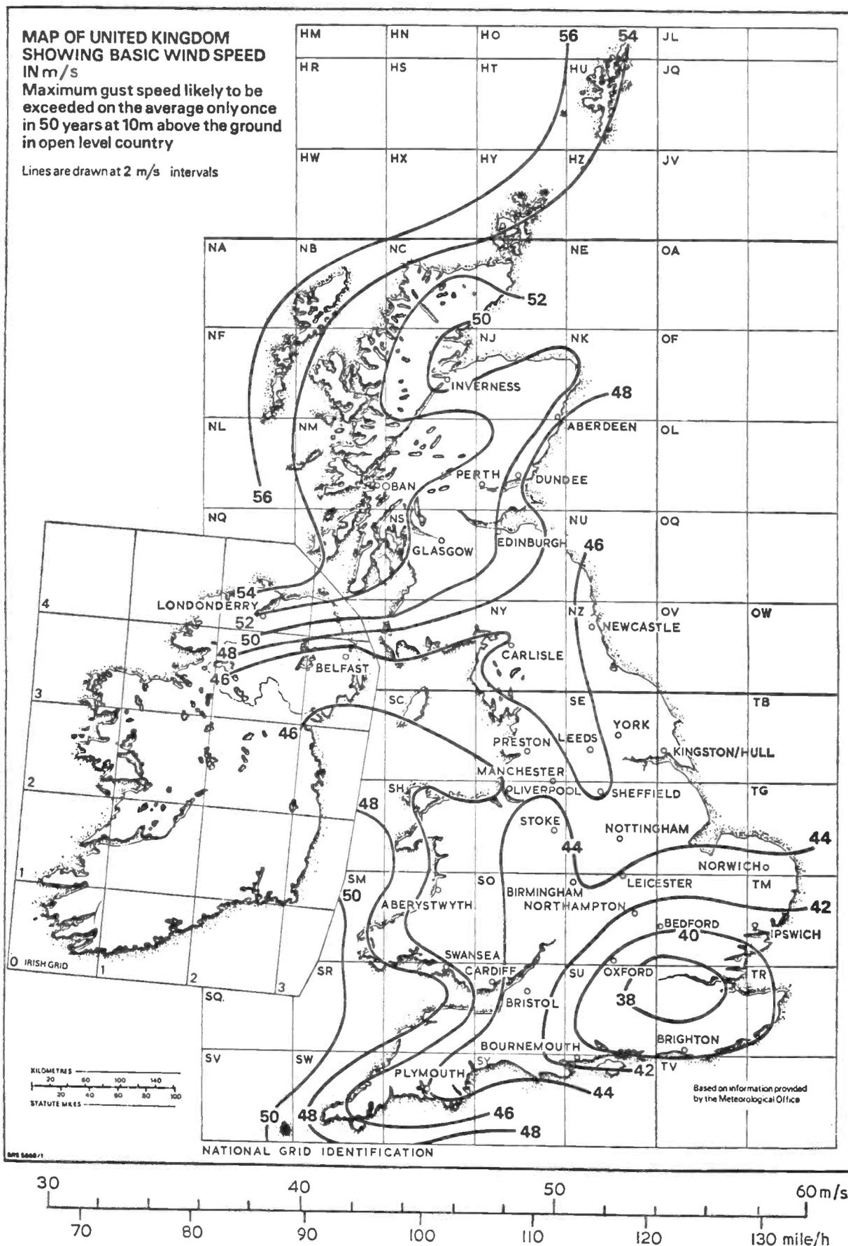
Fig. 1. Basic wind speed
