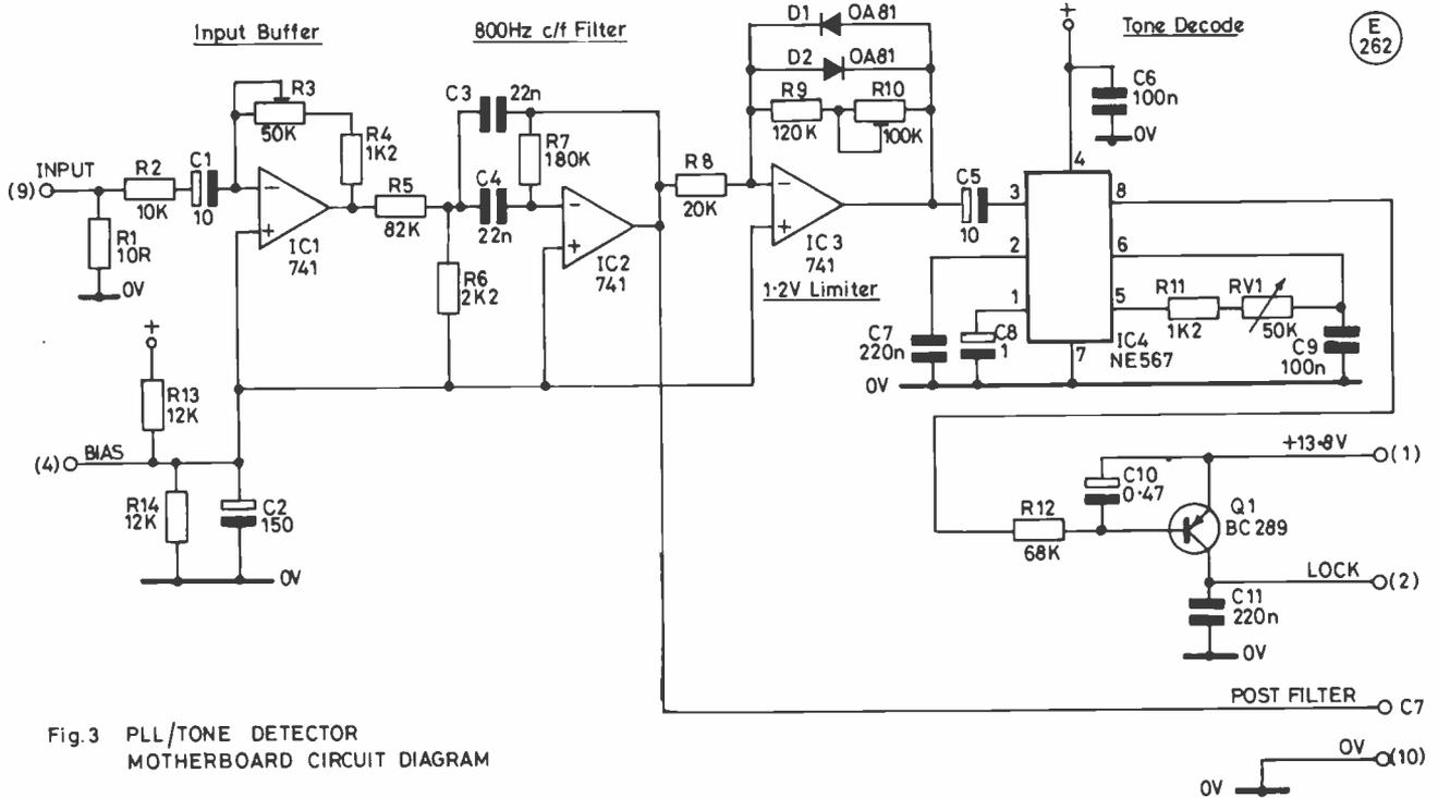
Fig. 3 PLL/TONE DETECTOR MOTHERBOARD CIRCUIT DIAGRAM
