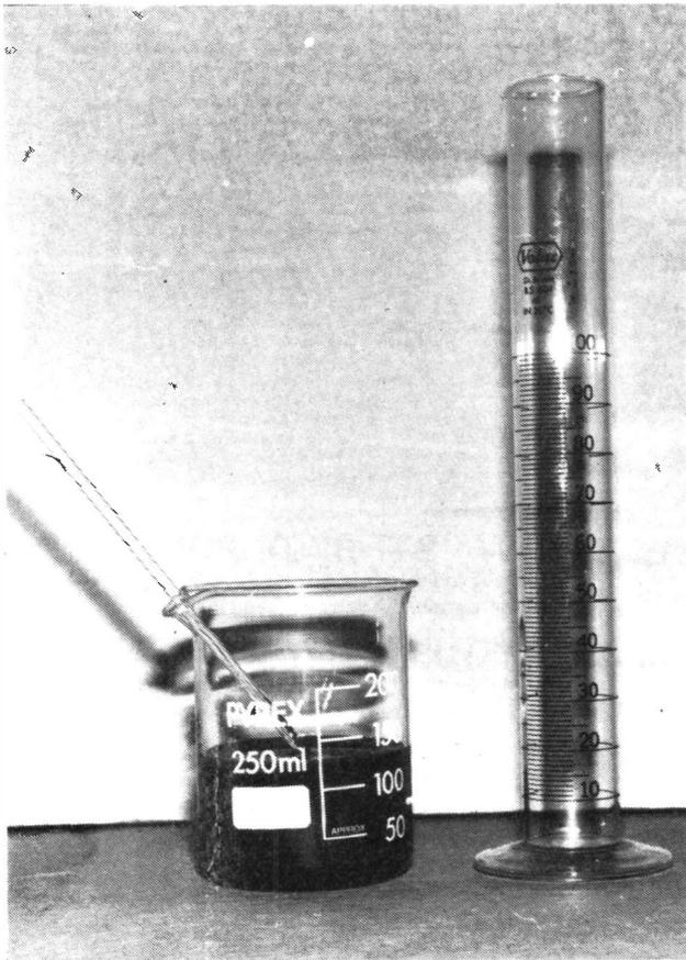
Fig. 4. The cylinder, glass rod and beaker containing the resin.
