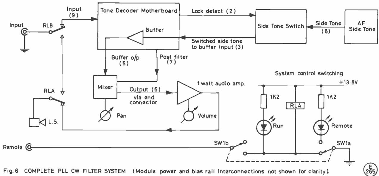
Fig. 6 COMPLETE PLL CW FILTER SYSTEM (Module power and bias rail interconnections not shown for clarity).
