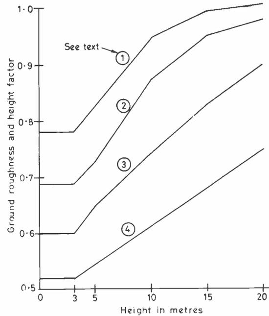
Fig. 2. Graph to determine value of ground roughness and height factor
