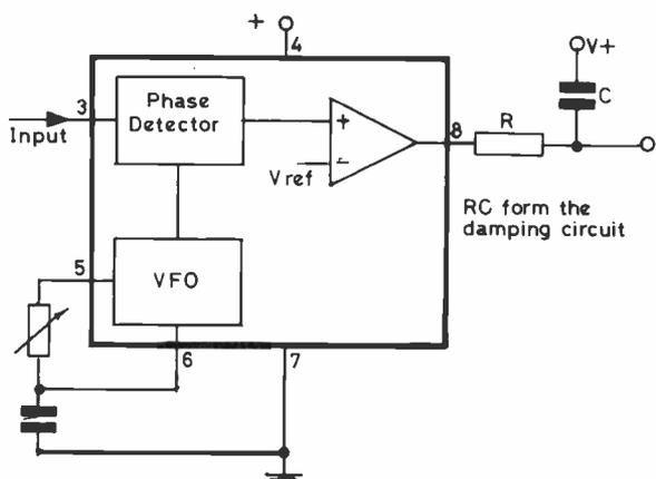
Fig.1 SIMPLIFIED BLOCK SCHEMATIC OF NE567 TONE DECODER/PLL
