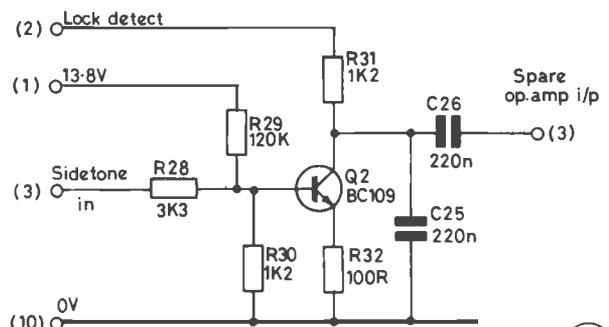
Fig.10a TONE SWITCHING MODULE CIRCUIT
