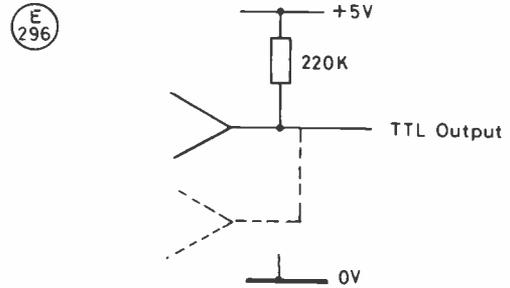
Fig.3 MODIFICATION FOR TTL LEVEL OUTPUT
