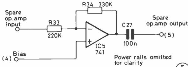
Fig. 11 BUFFER AMPLIFIER CIRCUIT.
