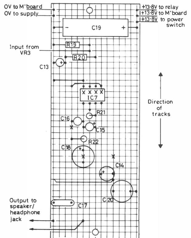
Fig.8b AUDIO POWER AMPLIFIER LAYOUT
