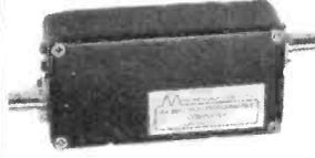
This low-noise converter when used in conjunction with a 28-30MHz receiver will provide reception of the 2 metre amateur band. All that is required is a 12 volt supply and a suitable antenna.
