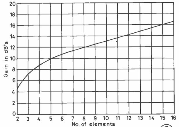
Fig. 2 Gain of array for number of elements
