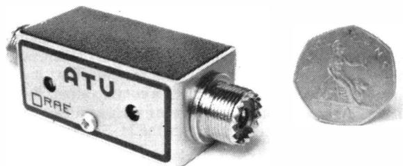
*Davtrend Ltd.* has come up with a new solution to the old problem of improving the VSWR of 2-metre mobile antennas. Shown here is the *DRAE* preset 2m. ATU which, when placed between antenna and transceiver, is claimed to give optimum performance for any given situation. The 30-watt, 50-ohm unit costs £11.80 inc. VAT, and full information is available from *Davtrend Ltd.*, Sanderson Centre, Lees Lane, Gosport, Hants. PO12 3UL. (Tel: Gosport 520141).
