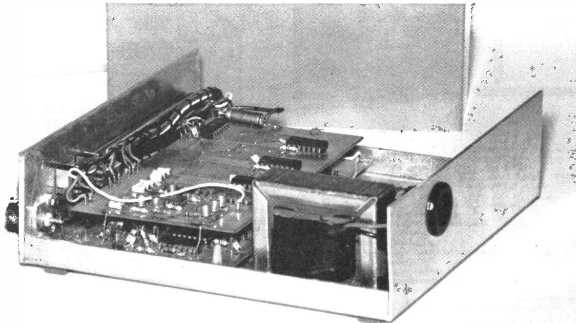
An inside view of the "Dover", showing both PCB's and transformer in position.
