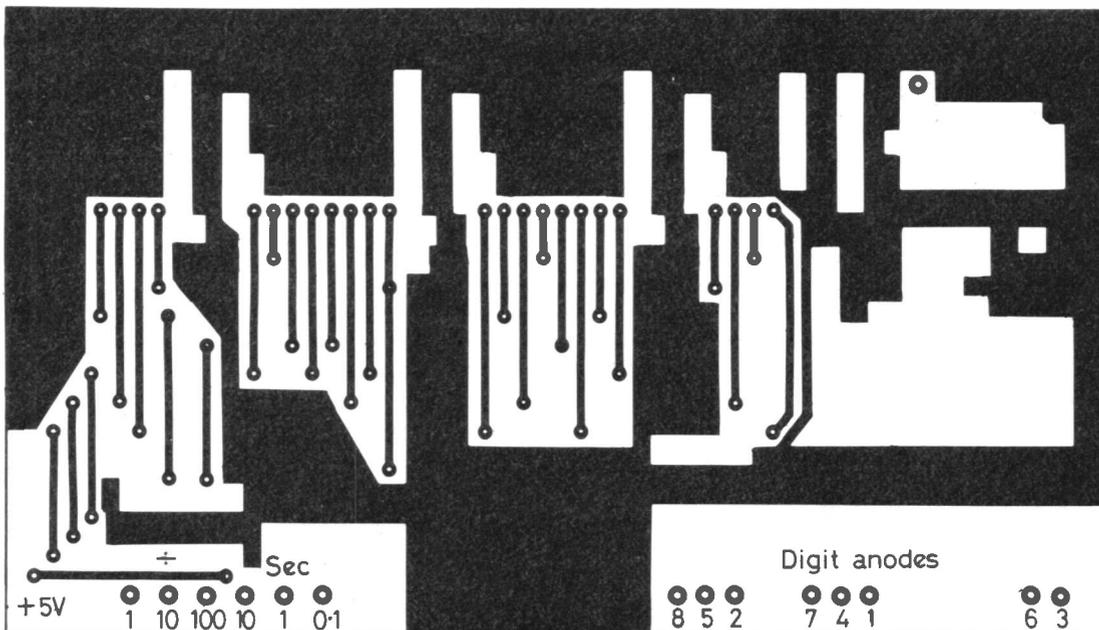
Fig.8 Decimal point Control PCB (top side)
