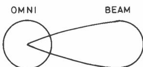
Fig. 1 Compares omni-directional and beamed “footprints”
