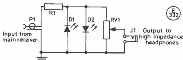
Fig. 2. Circuit of the Clipper / Limiter unit
