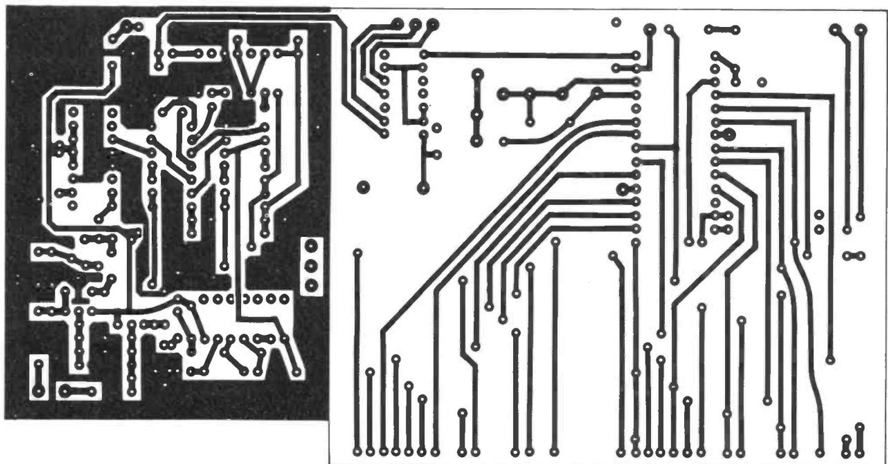
Fig. 5. 'Dover' Frequency Meter Prescaler and Counter PCB (underside).
