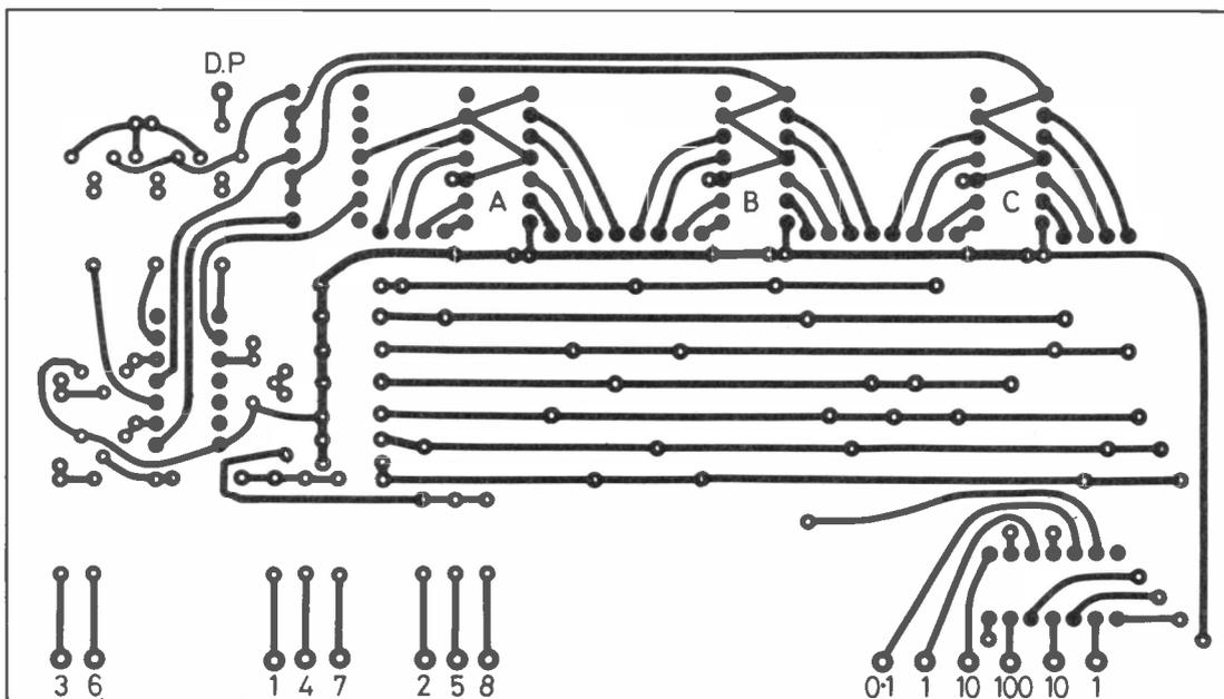
Fig.9 Decimal point Control PCB (underside).
