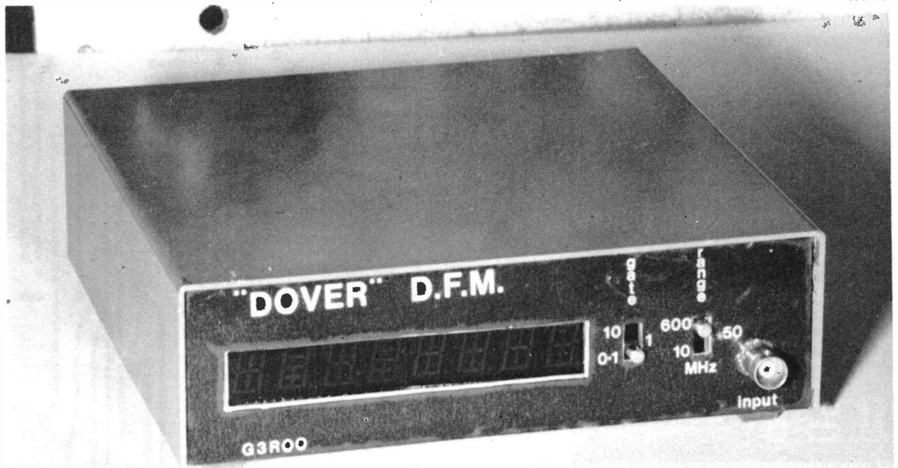
Front view of a completed "Dover" digital frequency meter.
