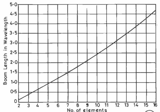
Fig. 3 Boom length versus number of elements
