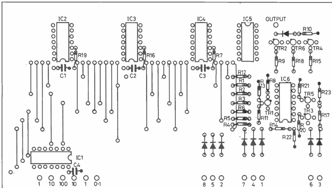
Fig.7 Decimal point Control PCB Component layout
