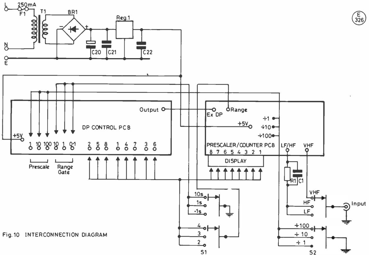
Fig. 10 INTERCONNECTION DIAGRAM
