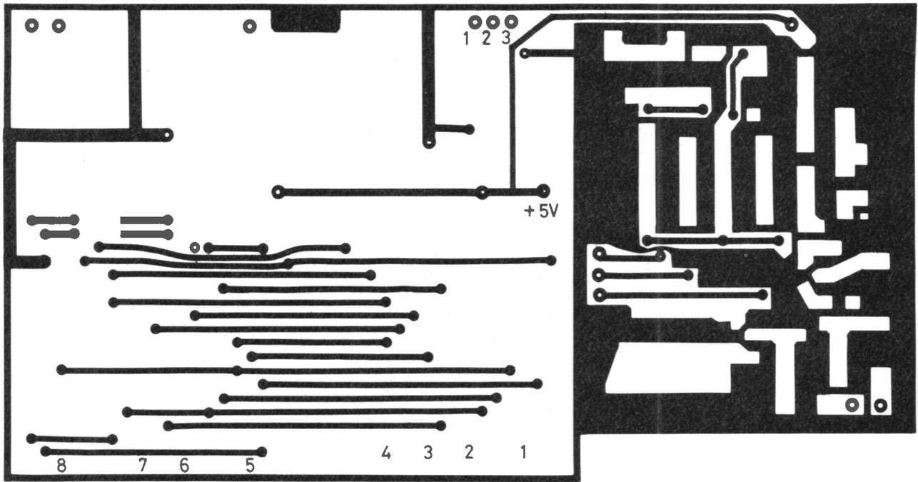
Fig.6 Prescaler and Counter PCB (top side)
