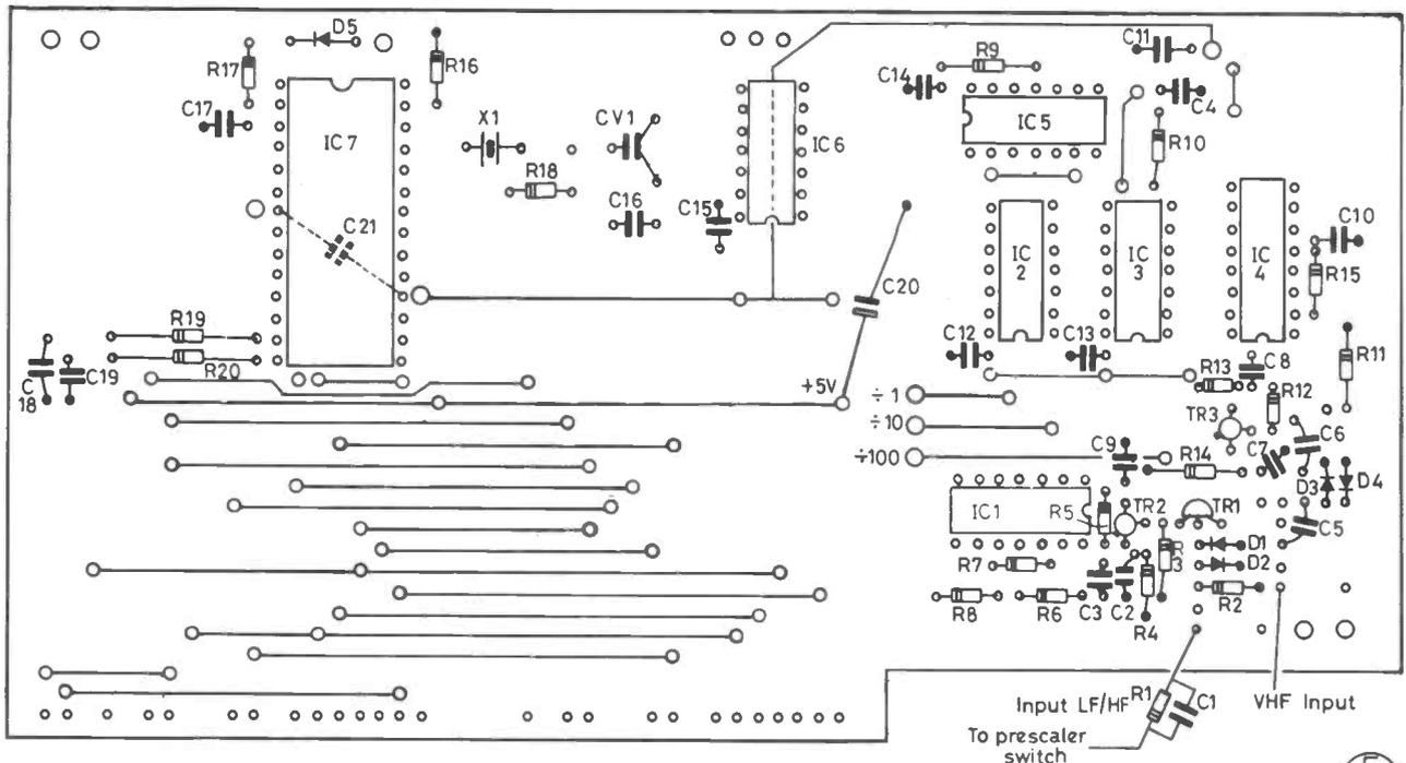
Fig. 4 Prescaler and Counter PCB Component layout
