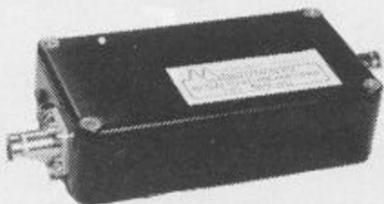
This RF switched low-noise receive pre-amplifier utilises the proven 3SK88 MOSFET in a noise matched design. Providing a power gain of 15dB and having a noise figure of 1.3dB, this unit will accept a through power of 100 watts.
