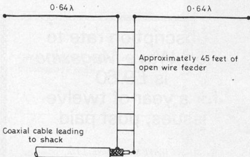
Fig. 1 Extended Double Zepp antenna for single band operation.
