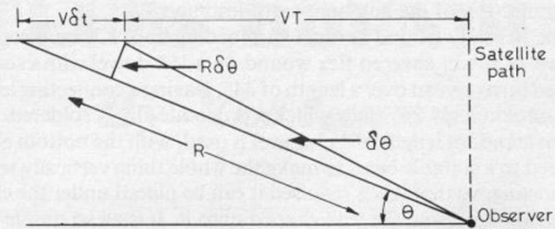
Fig.2 DOPPLER SHIFT OF TRANSMISSION FROM SATELLITE E
