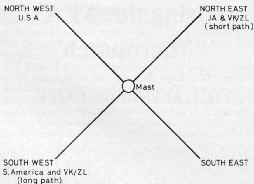
Fig. 4 The Full Sloper System looking from above showing the four best directions when using only four dipoles.
