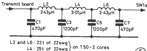
Fig. 2 LOW PASS FILTER
