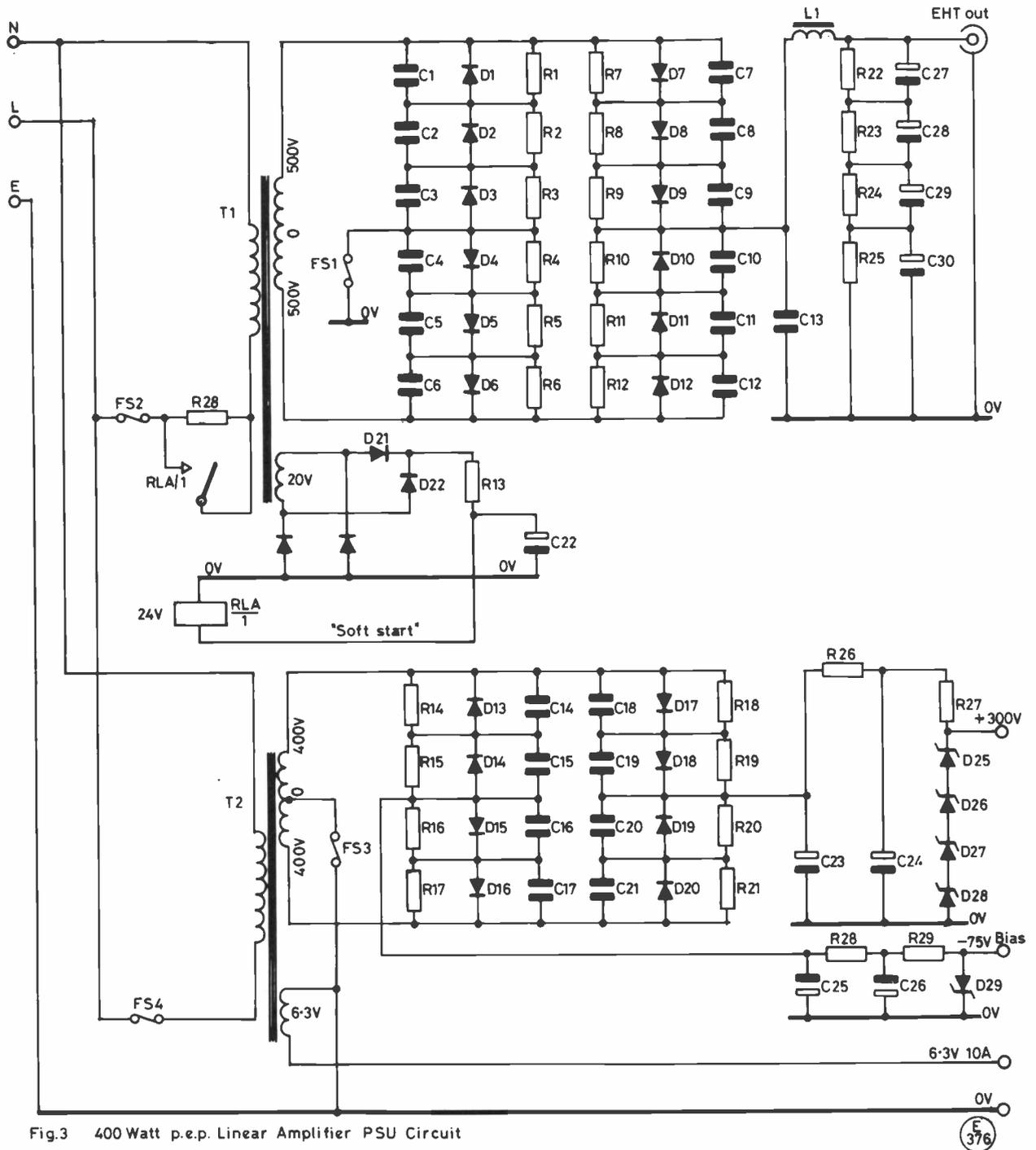
Fig.3 400 Watt p.e.p. Linear Amplifier PSU Circuit
