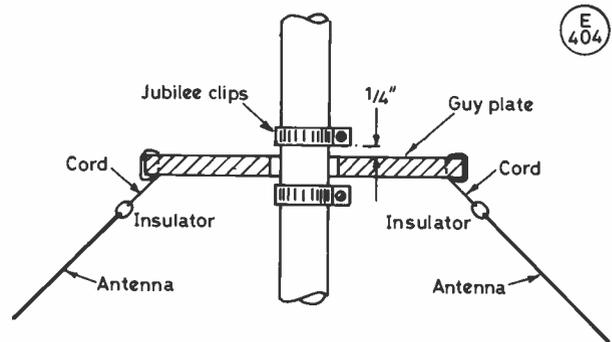
Fig.9 Diagram to illustrate a method of allowing a Sloper System to be attached to the top of a rotatable mast. The guy plate is one size too big for the mast.
