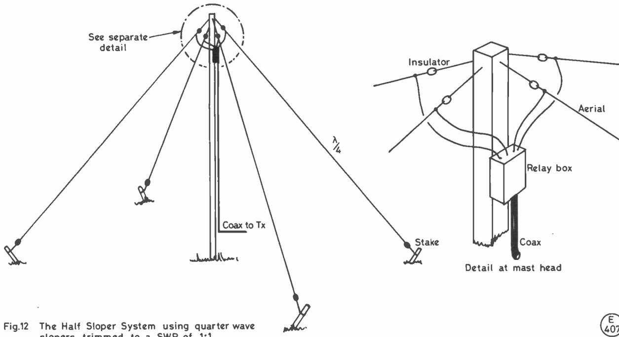
Fig.12 The Half Sloper System using quarter wave slopers trimmed to a SWR of 1:1
