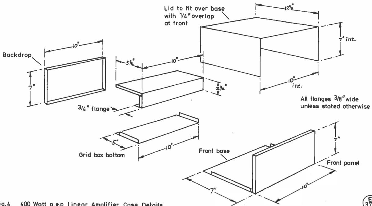
Fig. 4 400 Watt p.e.p. Linear Amplifier Case Details
