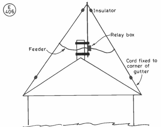
**Fig. 11** Full Sloper System for 14, 21 and 28MHz where there is insufficient space at the side of the house to hang the Sloper away from the roof.
