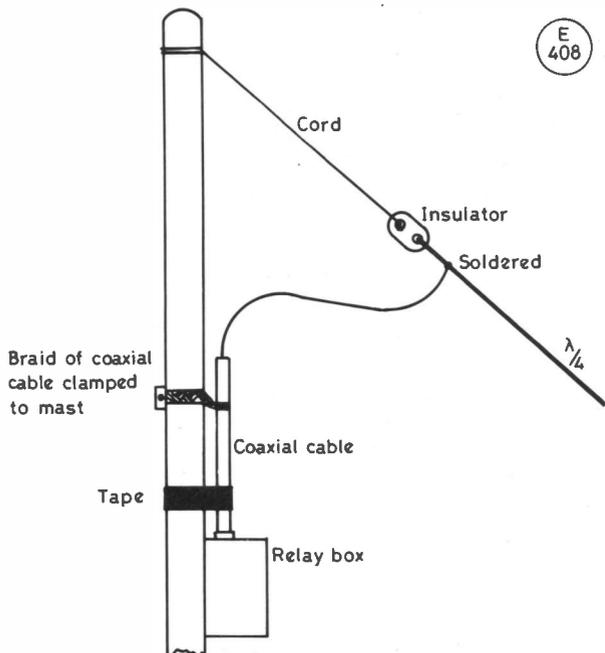
Fig.13 Connection of a 1/4 Sloper to the top of a mast
