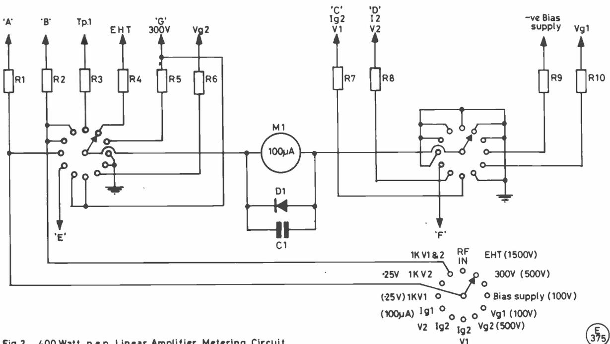
Fig.2 400 Watt p.e.p. Linear Amplifier Metering Circuit
