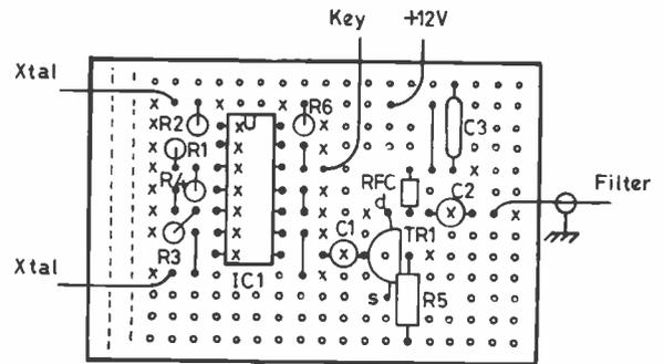
Fig.4 TRANSMITTER BOARD
