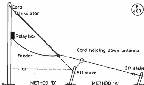
Fig.8 Showing two alternative ways of hanging the slopers. Method 'A' is where the ideal mast height cannot be achieved and Method 'B' where space prevents the slopers being stretched right out.
