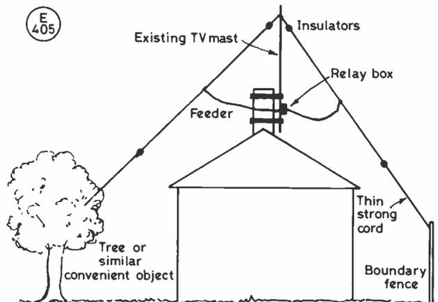
Fig.10 Full Sloper System for either 14, 21 or 28MHz installed on an existing TV mast with the slopers hanging towards each corner of the house. Two slopers only have been shown in the diagram.
