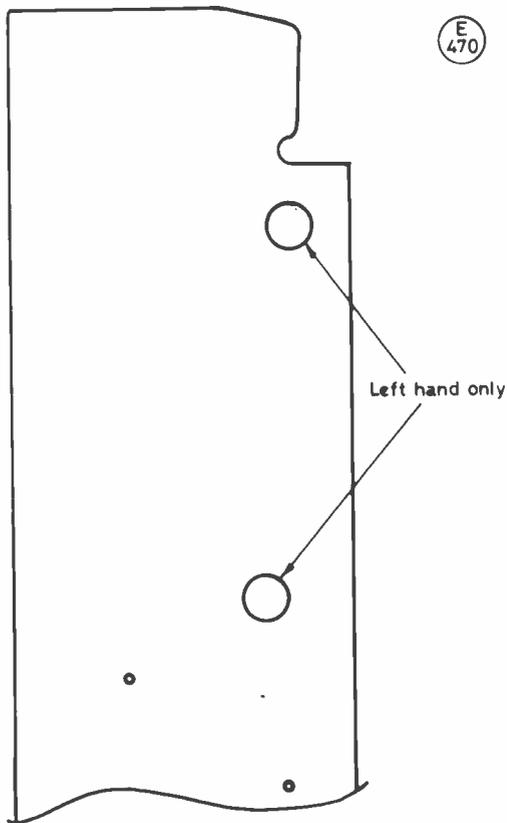
Fig. 5 TEMPLATE FOR FRONT END OF SIDES OF 'U' SECTION (Half full size).
