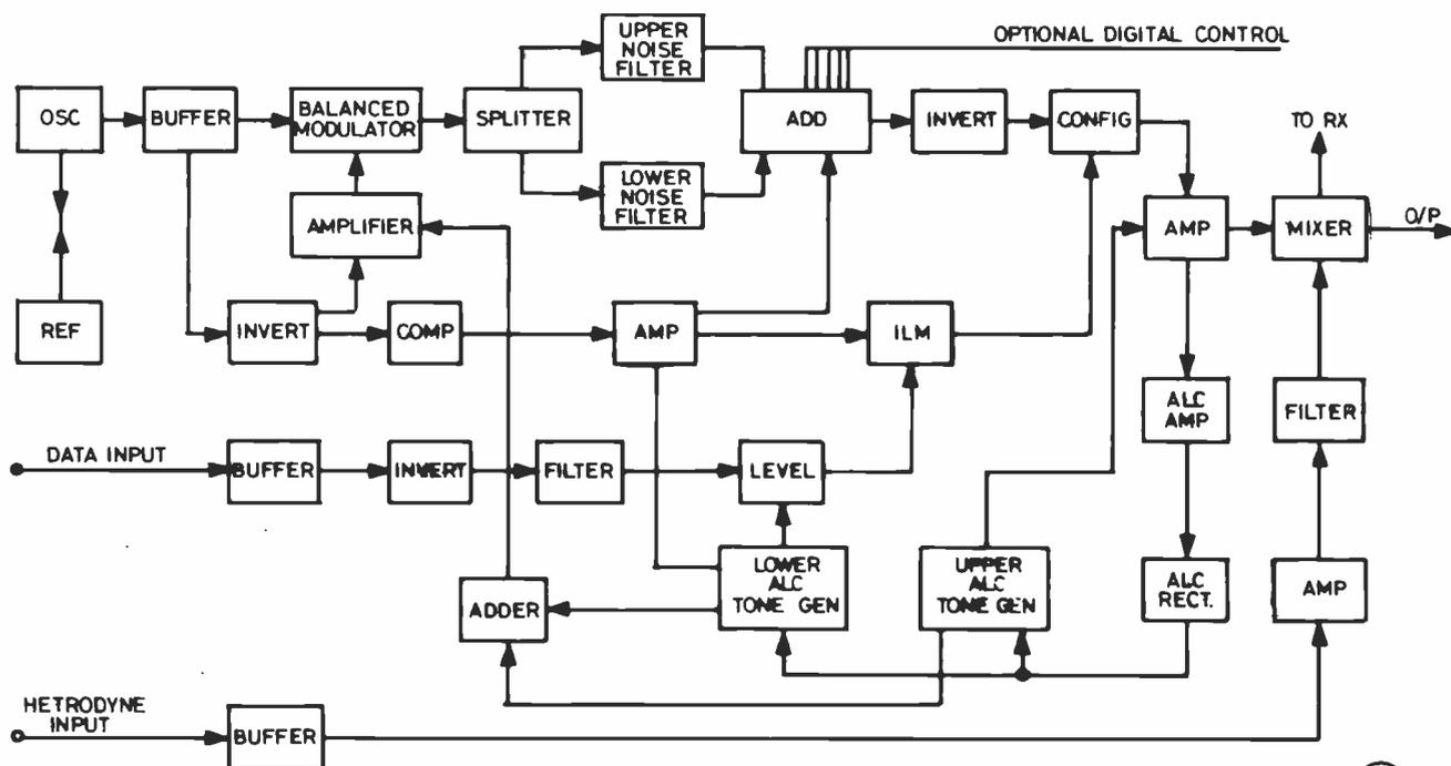
Fig.1 BLOCK DIAGRAM OF TRANSMITTER
