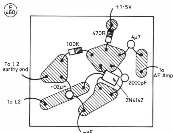
Fig.2 Plan view of the ZN414 Circuit Board
