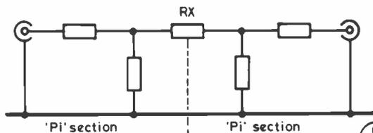
Fig.2 RX IS THE COMBINED VALUE OF TWO RESISTORS
