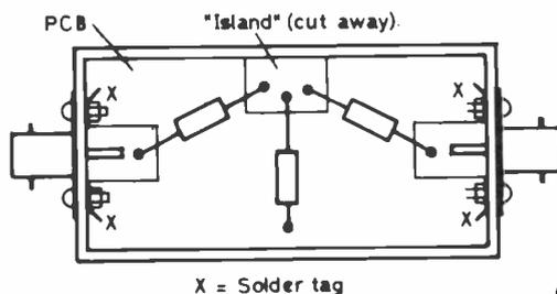
Fig.3 SINGLE STAGE ON "ISLAND" TYPE PCB
