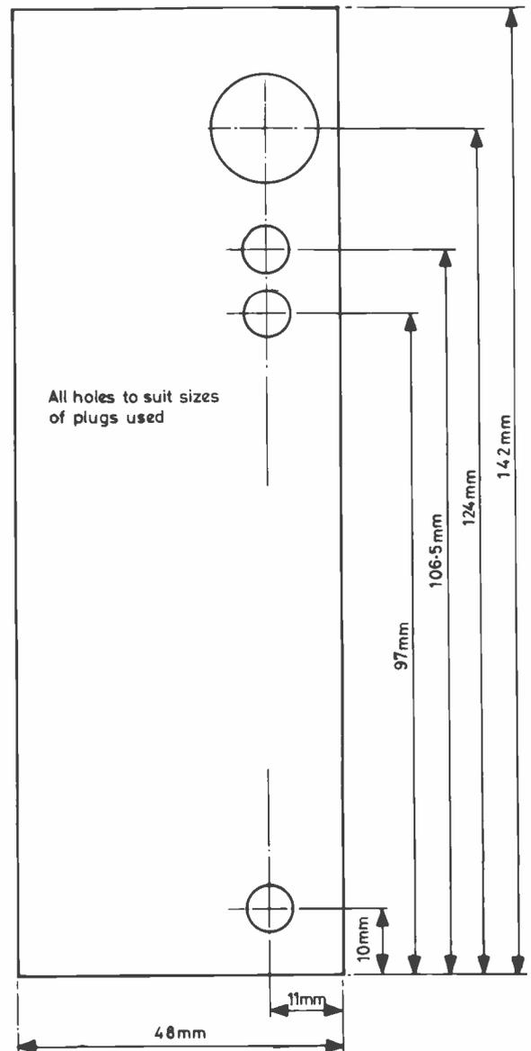
Fig. 6 TEMPLATE FOR PLUG ASSEMBLY (Full size)
