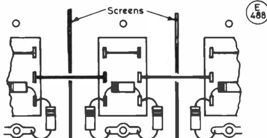
Fig.4 LAYOUT OF COMPONENTS FOR SWITCHED ATTENUATOR
