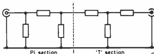
Fig.1 CASCADED 'Pi' AND 'T' SECTIONS
