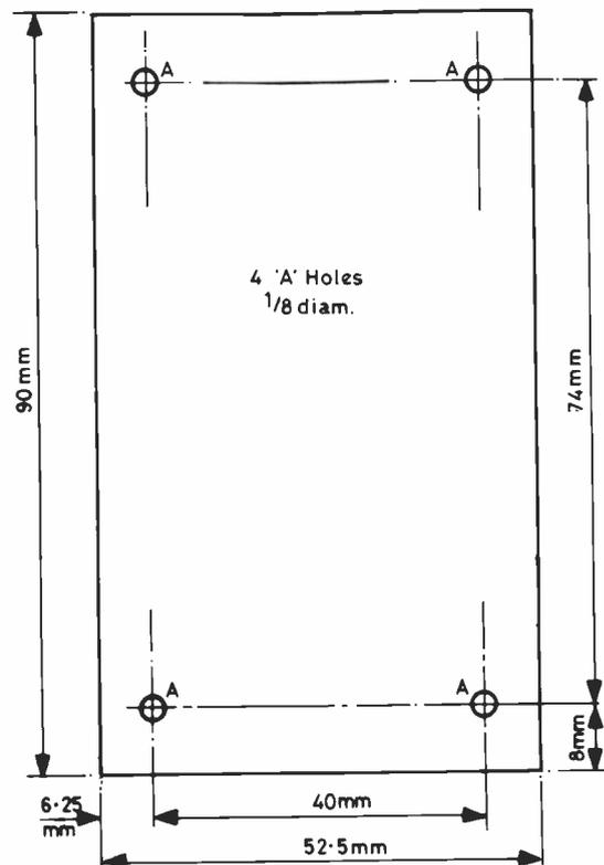
Fig. 6 DRILLING TEMPLATE FOR HOWES C.O.1 (Full size)
