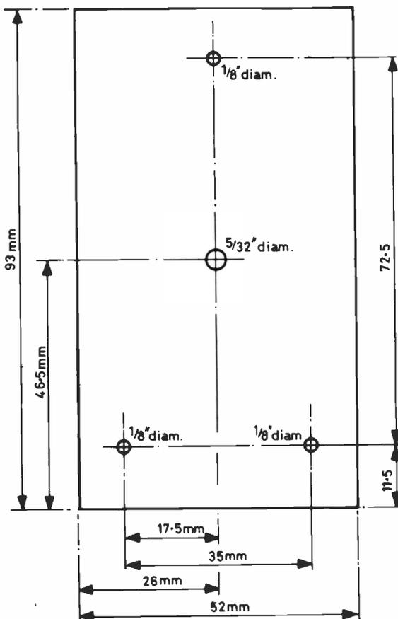
Fig. 7 DRILLING TEMPLATE FOR HOWES PA (Full size)
