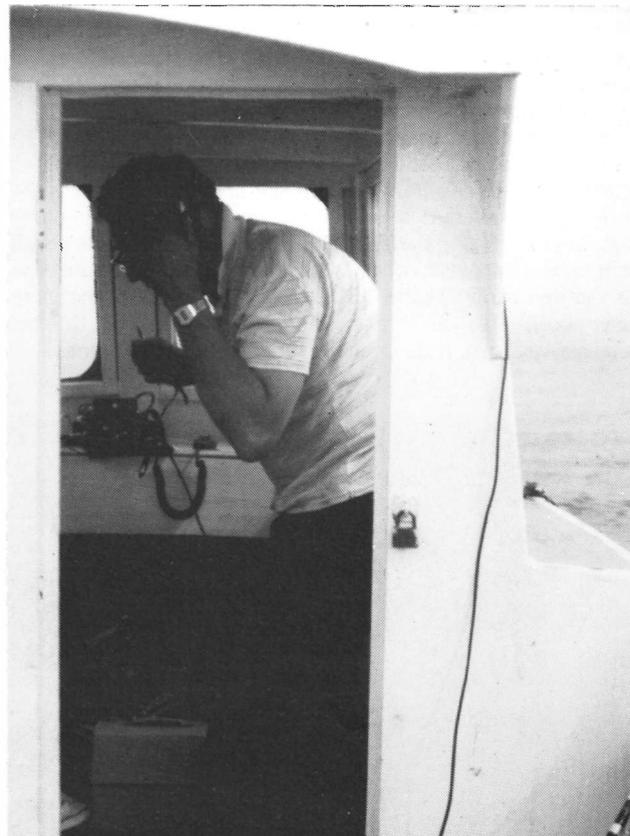
Bernard Atkinson operating G6EBH/MM in the wheelhouse of his diesel vessel *Prospect*. The transceiver is a Yaesu FT-290R with muTek front end. A Daiwa 30w amplifier is used with an HB9CV antenna for SSB and a  $\frac{1}{8}$ -wave vertical for FM/repeaters. The boat is 22ft. long and 8' -6" beam with a 12½ h.p. main engine and a 7½ h.p. auxiliary. Listen for G6EBH/MM on summer weekends and sometimes on Wednesday afternoons from AO square on 2m.
