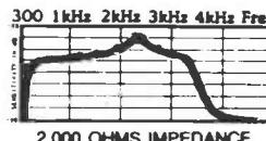
The element works very well into a 600 ohm load, but it may need a matching transformer when using high impedance outputs.
