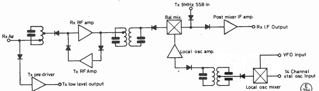
Fig. 2 BLOCK DIAGRAM FT707 RF PCB (Diodes indicate diode switches).
