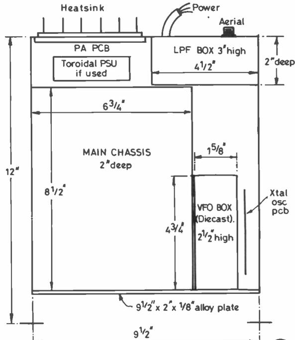
Fig. 7 Main Chassis Layout
