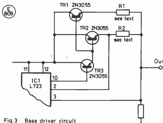
Fig. 3 Base driver circuit
