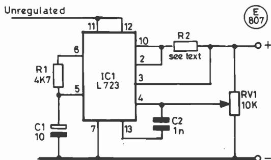
Fig. 1 Basic regulator with current limit
