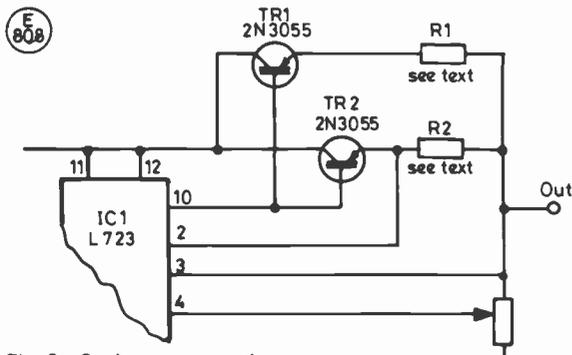
Fig. 2 Series pass section
