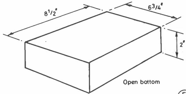
Fig. 8 Main chassis box (16 swg alloy)
