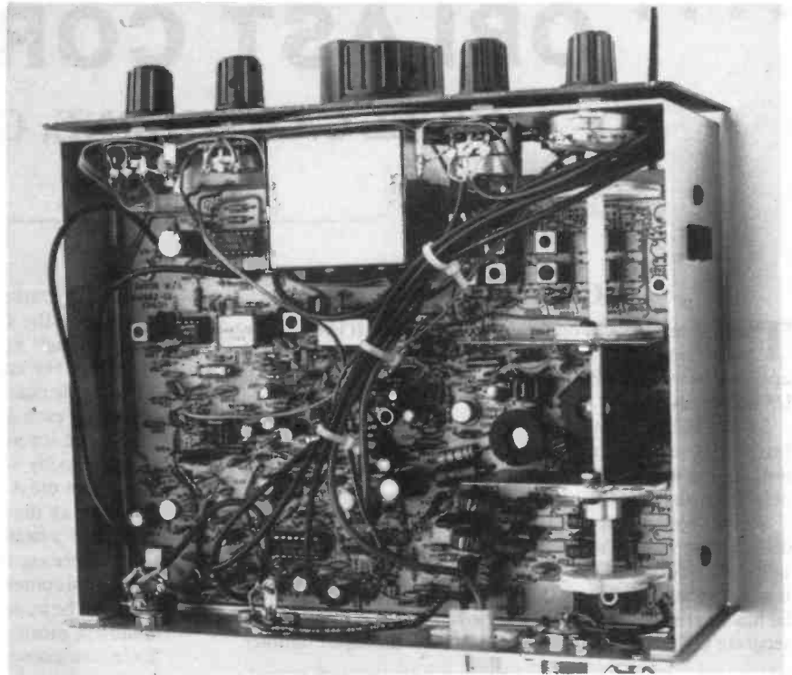
Bottom view of the HW-9 showing the receive PCB.
