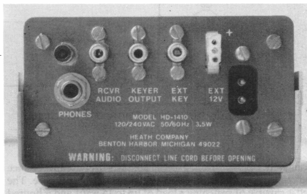
Rear view of the modified keyer showing the additional phono socket at upper left.
