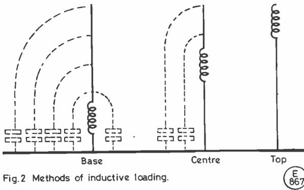
Fig.2 Methods of inductive loading.
