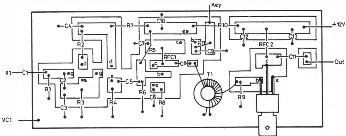
Fig. 2 S.C.D. Mk.II LAYOUT - FULL SIZE (Copper side up)
