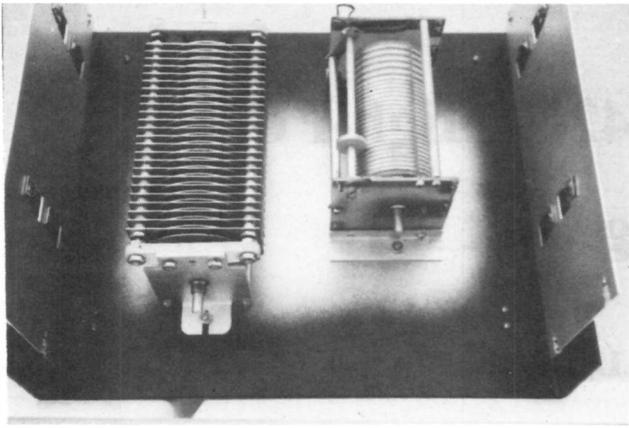
Showing assembled variable capacitor and inductor. Note the position and mounting of the side panels.
