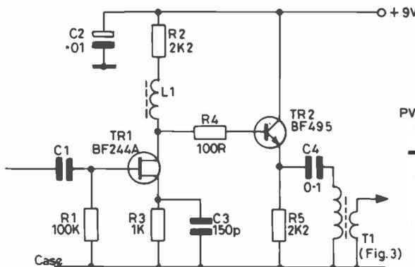
Fig. 2 PROBE CIRCUIT DIAGRAM
