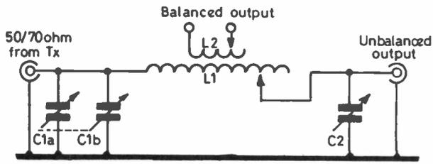
Fig. 4 A Z-match type of matching unit suitable for use with low impedance balanced loads. This circuit also works well with a wide range of unbalanced loads. E 859
