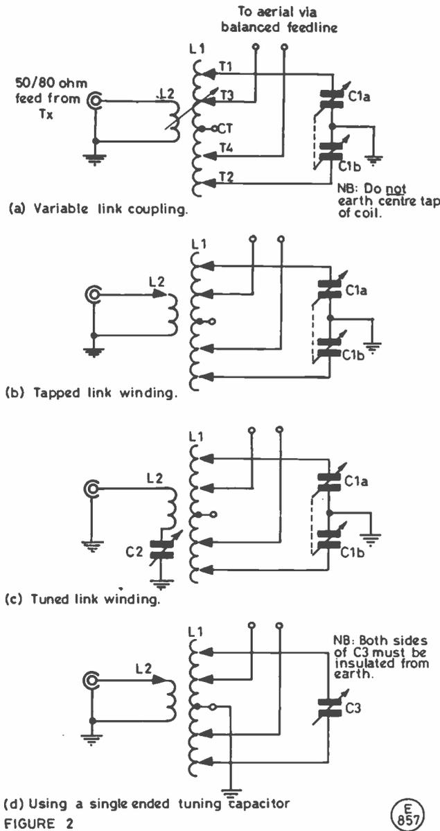
Fig. 2: The link coupled parallel-tuned matching unit for use with balanced feeders showing: (a) variable or 'swinging' link coupling; (b) a tapped link winding; (c) a tuned link winding; (d) the use of a single-ended tuning capacitor.
