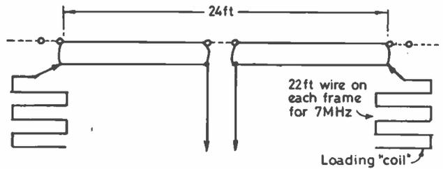
(a) 'Open' inductive loading of the loft mounted dipole for 7MHz operation as described in text.
