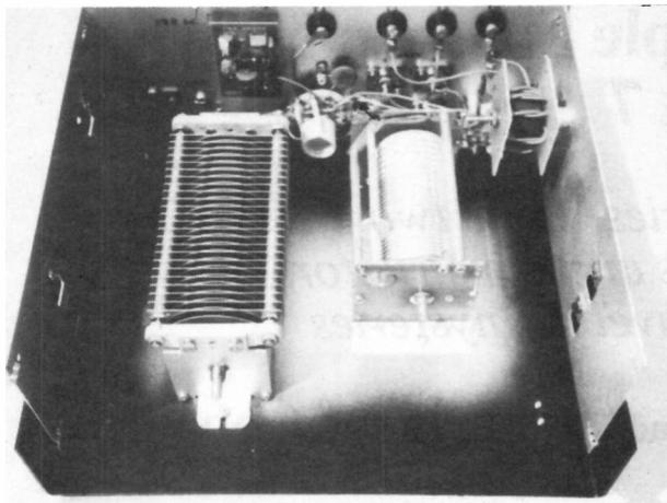
Rear panel in position. Note SWR board above variable capacitor and balun in right corner.
