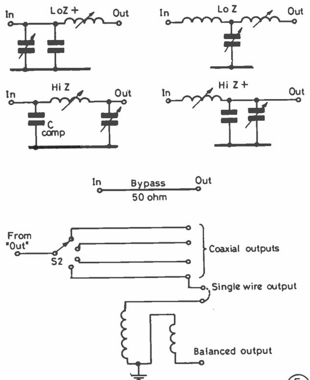
Fig. 1 TUNER CONFIGURATIONS (Selected by S1)
