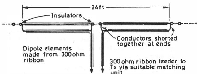
1a. Loft mounted 14-28 MHz aerial used at DA1PE
