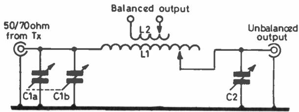
Fig. 4 A Z-match type of matching unit suitable for use with low impedance balanced loads. This circuit also works well with a wide range of unbalanced loads. E 859
