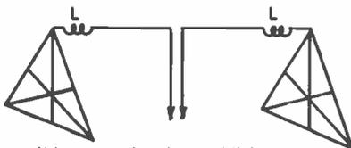
(c) One possible way of using additional lumped inductive loading for lower frequency operation
