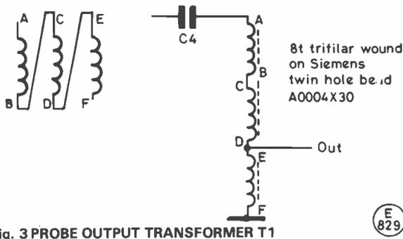
Fig. 3 PROBE OUTPUT TRANSFORMER T1
