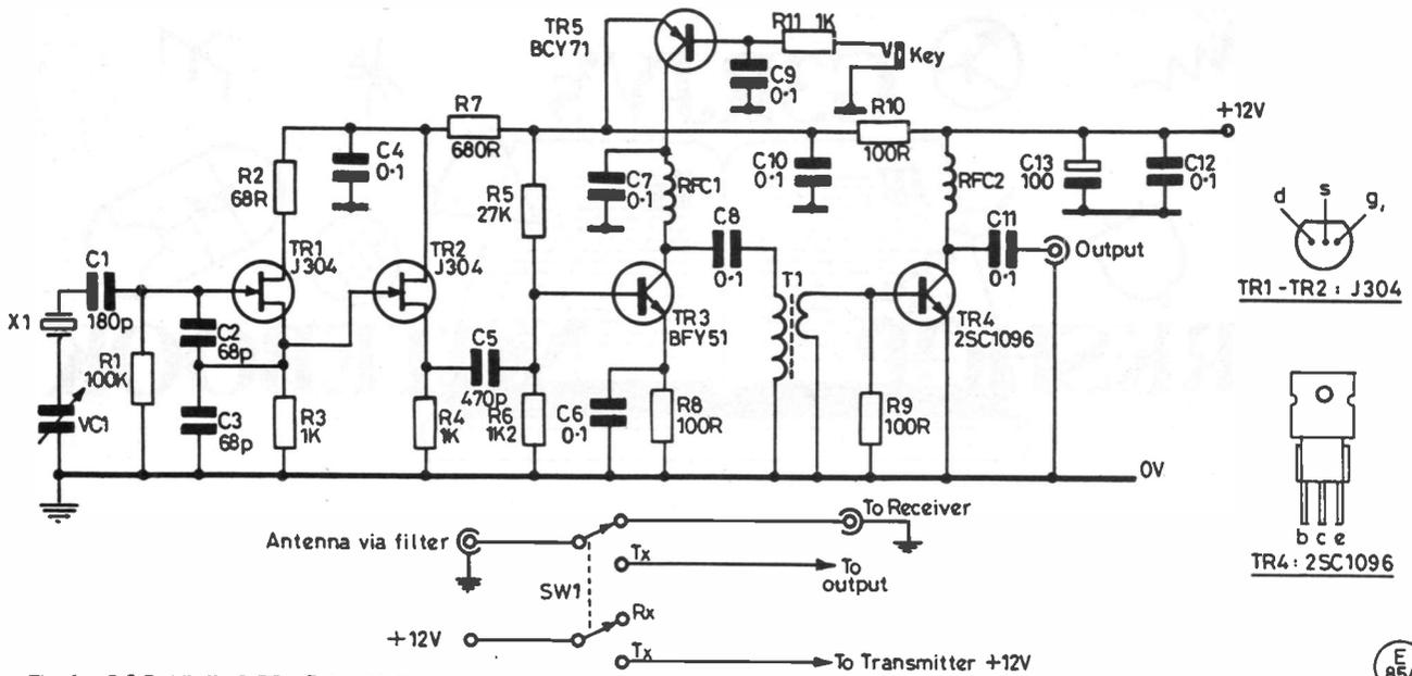
Fig.1 S.C.D. Mk II CIRCUIT DIAGRAM
