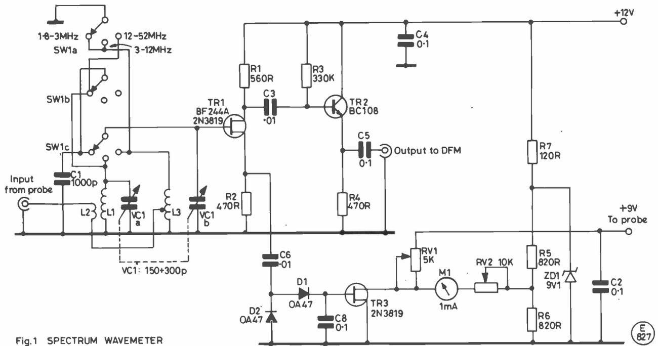
Fig. 1 SPECTRUM WAVEMETER
