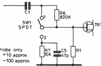
Fig. 4 PROBE SWITCHED ATTENUATOR
