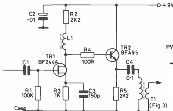
Fig. 2 PROBE CIRCUIT DIAGRAM
