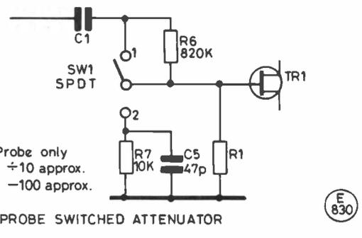
Fig. 4 PROBE SWITCHED ATTENUATOR
