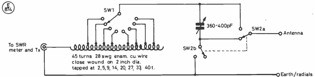
Fig. 6 L-MATCH and SERIES TUNED A.T.U. for END FED ANTENNAE.
