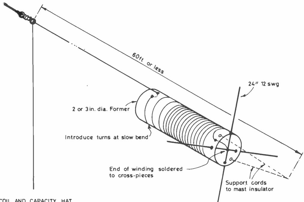
Figure 5. DETAIL OF COIL AND CAPACITY HAT
