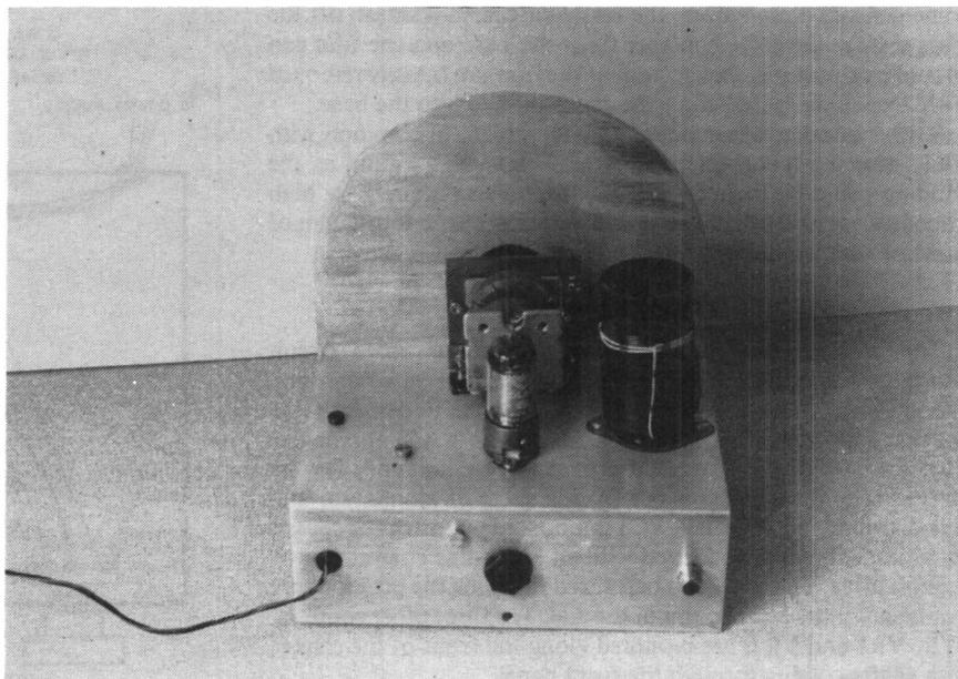
used electron coupled feedback for regeneration, which does away the need for a variable capacitor as a reaction control. I sought and found the circuit and began to play about with versions of it.
