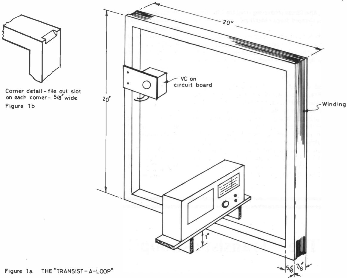
Figure 1a THE "TRANSIST-A-LOOP"
