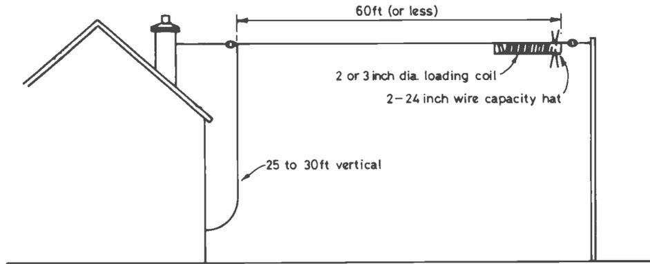
Fig. 4 BASIC LAYOUT OF THE COIL-LOADED INVERTED L
