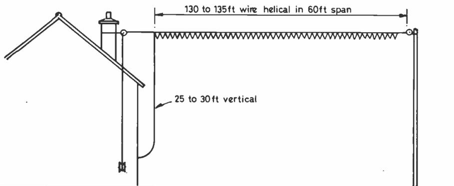
Fig. 3. BASIC LAYOUT OF THE INVERTED L HELICAL
