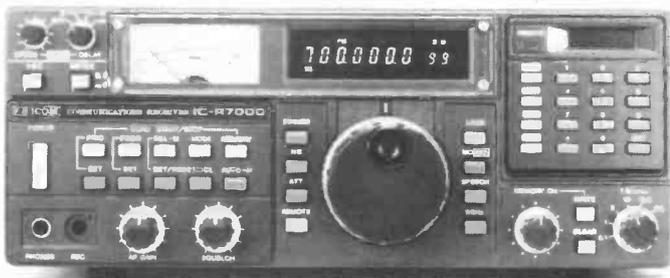
Other features include dial-lock, noise blanker, attenuator, display dimmer and S meter and optional RC-12 infra-red remote controller, voice synthesizer and HP1 headphones.
