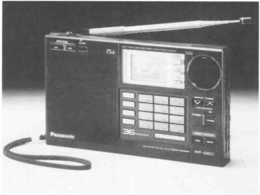
The clock is displayed when the set is switched off, or may be shown during operation by depressing the appropriate key. Dual time is recalled by the operation of a further button.
