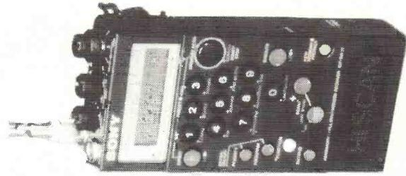
The long, medium and short wave bands all utilise dual-conversion superheterodyne techniques with the extremely high 1st i.f. of 55.845MHz realised by the high selectivity monolithic crystal filter.
