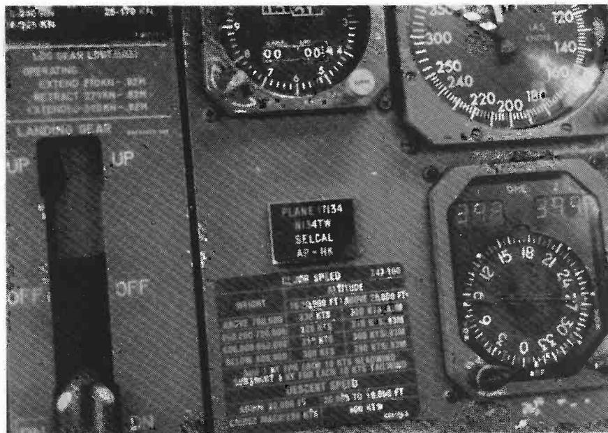
You can see the number of the aircraft and its SELCAL from the plate on the control panel.
