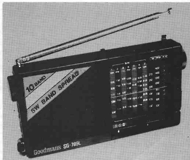
about 5% out, but this is not uncommon on a portable receiver. As the broadcast bands are covered in seven segments the main tuning becomes more akin to a bandspread dial. This greatly eases tuning on the very congested band conditions found after dark.
