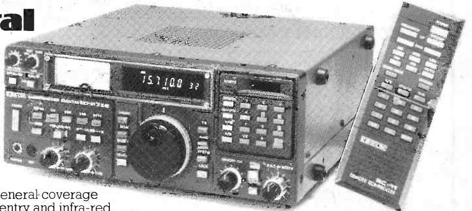
The ICOM IC-R71E 100KHz to 30MHz general coverage receiver features keyboard frequency entry and infra-red remote controller (optional) with 32 programmable memory channels, SSB, AM, RTTY, CW and optional FM. Twin VFO's scanning, selectable AGC, noise blanker, pass band tuning and a deep notch filter. With a direct entry keyboard frequencies can be selected by pushing the digit keys in sequence of frequency. The frequency is altered without changing the main tuning control.
