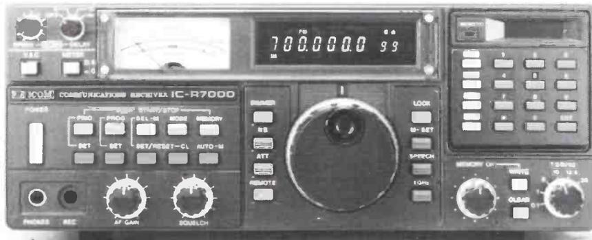
ICOM introduces the IC-R7000, advanced technology, continuous coverage communications receiver. With 99 programmable memories the IC-R7000 covers aircraft, Marine, FM Broadcast, Amateur Radio, television and weather satellite bands. For simplified operation and quick tuning the IC-R7000 features direct keyboard entry. Precise frequencies can be selected by pushing the digit keys in sequence of the frequency or by turning the
