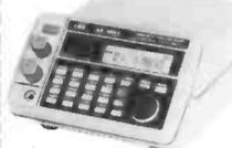
The frequency range is from 25 to 550 and from 800 to 13000MHz. Modes of operation are wide band FM, narrow band FM and AM. The receiver has 20 memories, memory scan and a search mode which checks frequencies between user designated limits and a push button keypad for easy frequency entry and operation. A front panel knob allows the listener to quickly step up or down in either 5, 12.5 or 25kHz steps from the frequency initially chosen.
