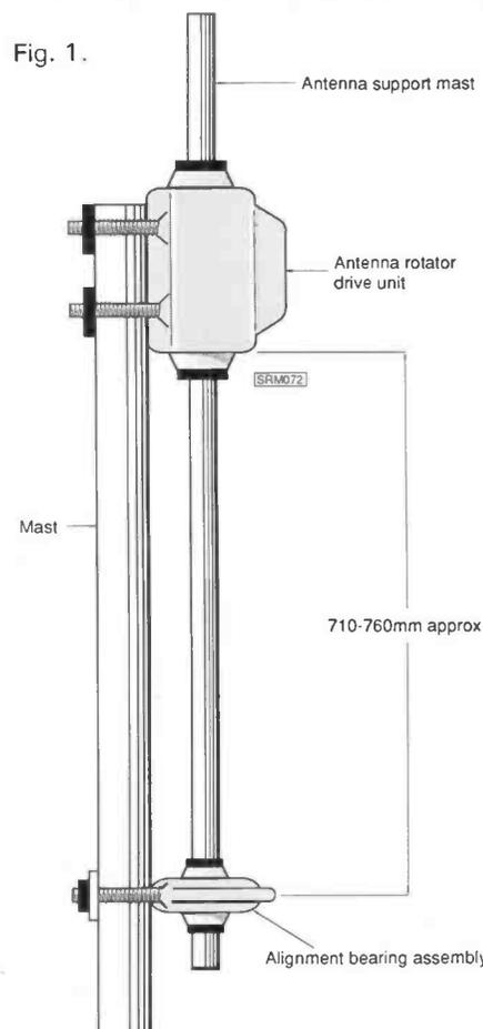
cannot be guyed since this would impede antenna rotation. Therefore, the weakest part of the structure will be immediately above the upper guy clamps. In many systems, this is usually where the antenna support pole enters the rotator.
