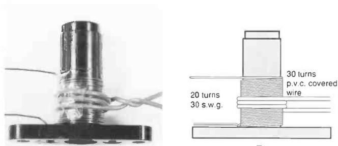
Fig. 3.4: Winding details for T1.
