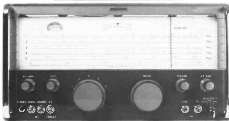
With the covers in place, connect up the receiver and run it for an hour or so with a towel covering the air vents. Keep an eye on it as the temperature will rise dramatically! If any component is likely to fail it will do so under these conditions. Switch off and allow to cool for a couple of hours, repeat the cycle and correct any faults that may have shown up.
