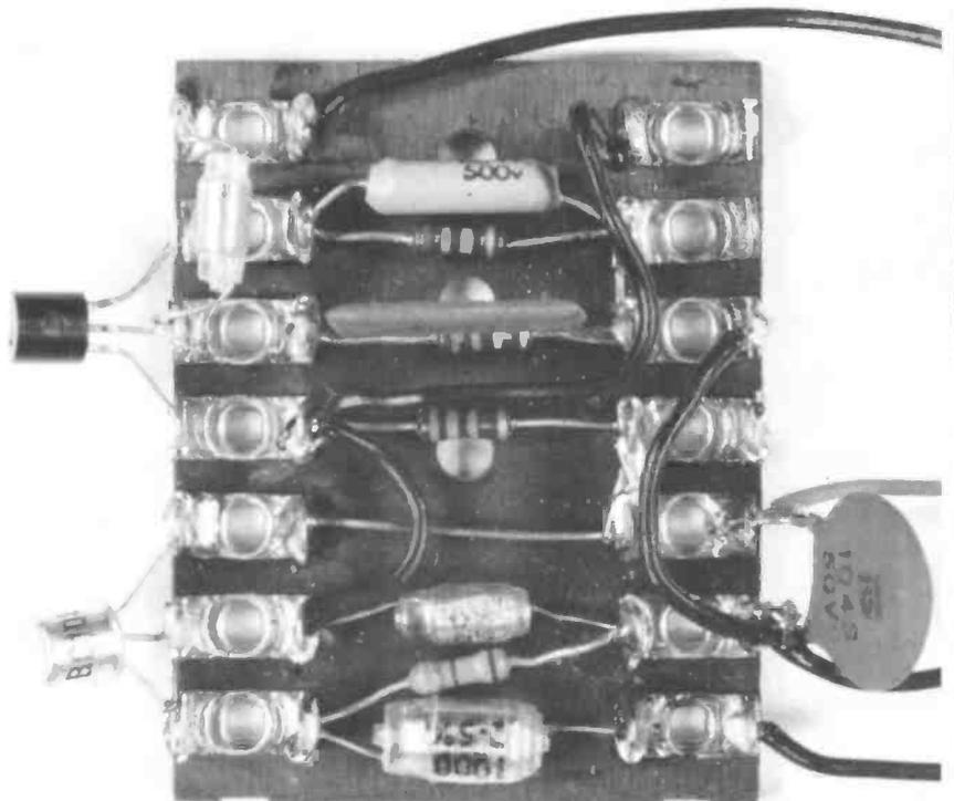
Fig. 3.2. Completed v.f.o. board.
