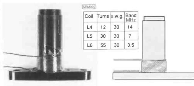
Fig. 3.3: Coil winding details.
