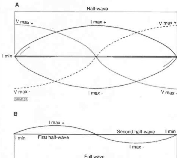
Fig. 1.1. (a) current and voltage distribution on a half-wave antenna; (b) current distribution on two half-wave antennas, i.e. full-wave antenna (see text).
