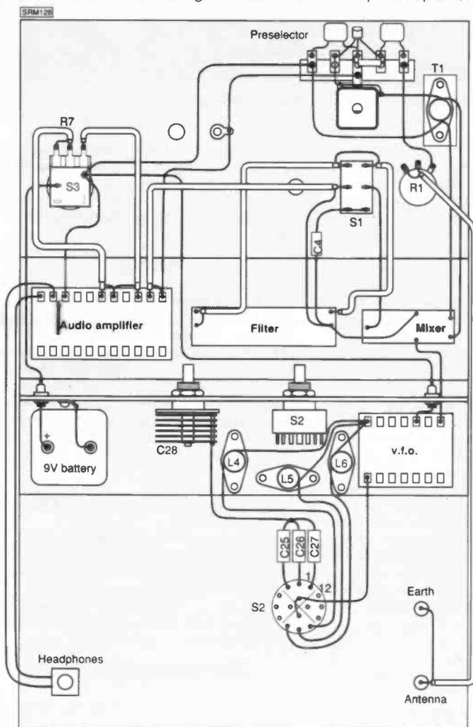
Fig. 6.1: The complete wiring diagram of the 3-Band s.s.b. Receiver. Note that the front and back panels are shown laid flat for clarity. The band selector switch, S2, has been shown removed from its correct position on the intermediate panel so that the connections to it can be shown correctly. In Fig. 5.1 the coils L4, 5 & 6 and T1 were shown incorrectly as L2, 3 & 4 and L1 respectively. These have been corrected in this drawing.
