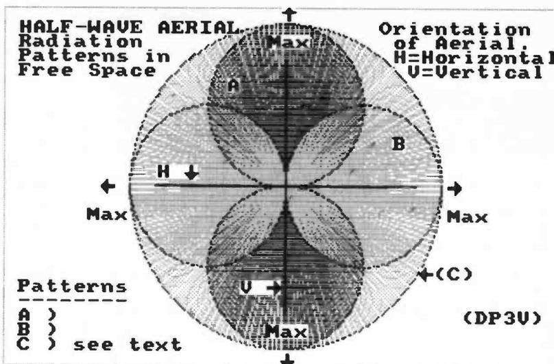
Fig. 1.4. (Above) Radiation patterns from a  $\lambda/2$  (dipole) antenna (see text).
