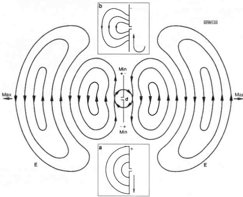
Fig. 1.3. Simplification of how radiation occurs from a  $\lambda/2$  antenna; it can be seen that a distinct pattern is emerging (see Fig. 1.4).
