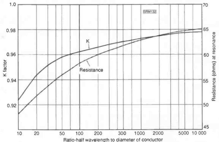
Fig. 1.2. Graph to obtain the "K" factor from the ratio of a half-wavelength to conductor-diameter; the average "K" factor is 0.95.
