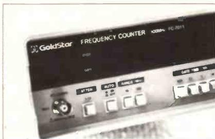
year. The models 7012 and 7013 are both fitted with temperature compensated crystal oscillators with better than 1 p.p.m. temperature stability and ageing rate per year. The case material for the 7012 is ABS plastics and aluminium for the 7013. The 7011 model costs £98 excluding VAT.
