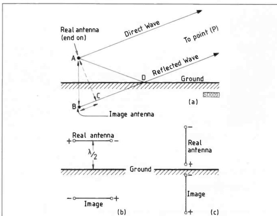
Fig. 3.1: (a) function of ground reflection; (b) the "image" antenna theory, (see text).
