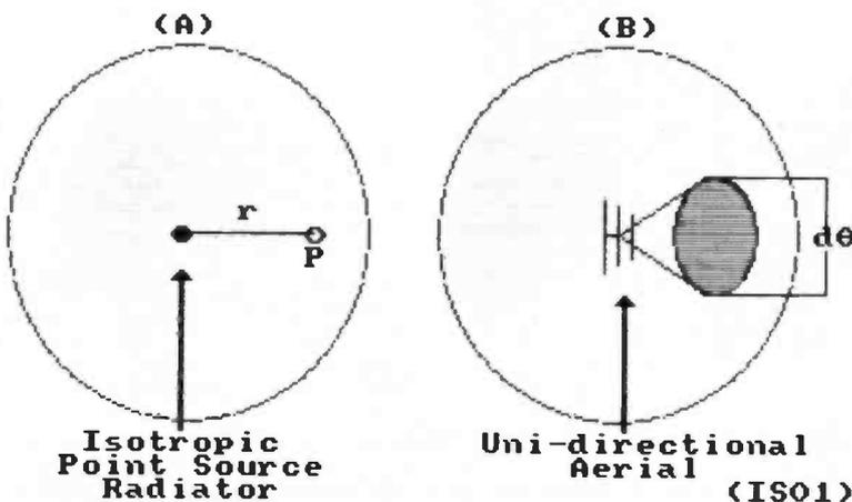
**Fig. 3.3: The isotropic (point source) radiator. Annotations & text describe the theory.**
