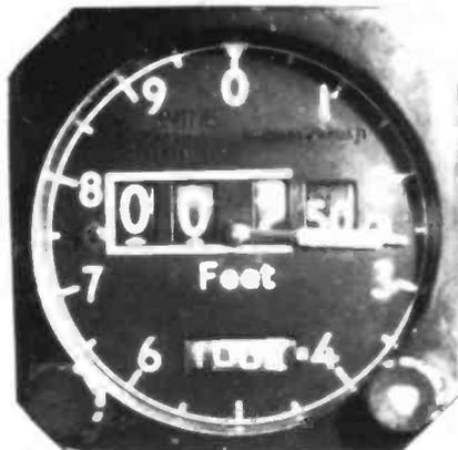
Fig. 2: QNH set to 1004mb. On the ground, altimeter reads airfield elevation of 267ft.
