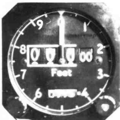
Fig. 1: QFE set to 995mb. On the ground altimeter reads zero feet.
