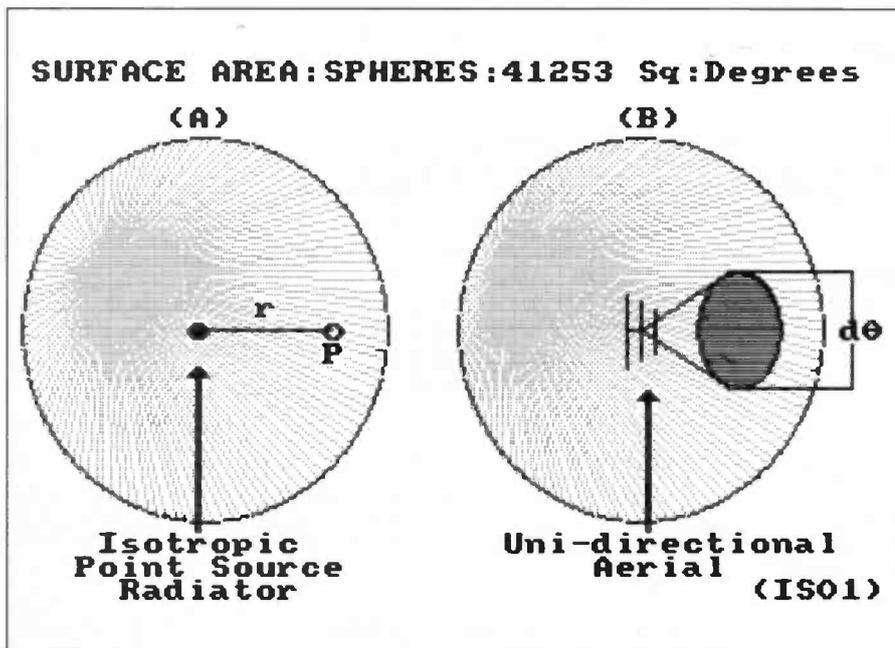
Fig. 4.1: The isotropic (point source) radiator. Annotations and text describe the theory.
