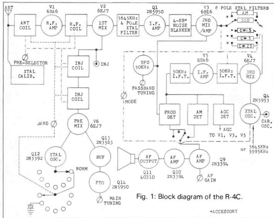
Fig. 1: Block diagram of the R-4C.
