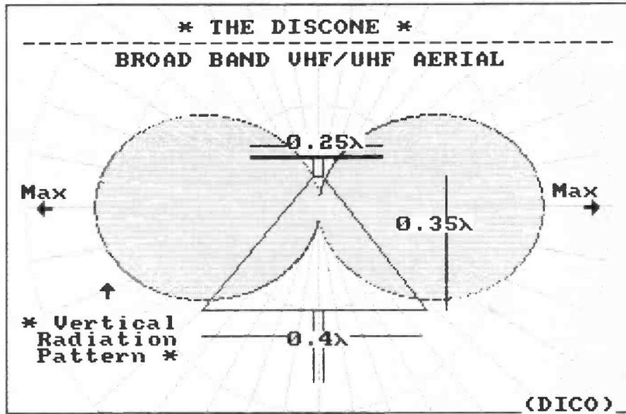
Fig. 6.2: Typical vertical radiation pattern and dimensions for a discone antenna.
