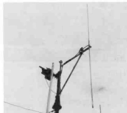
Fig. 6.5. Prototype of 2-element collinear with extended half-wave element spacing, see text.
