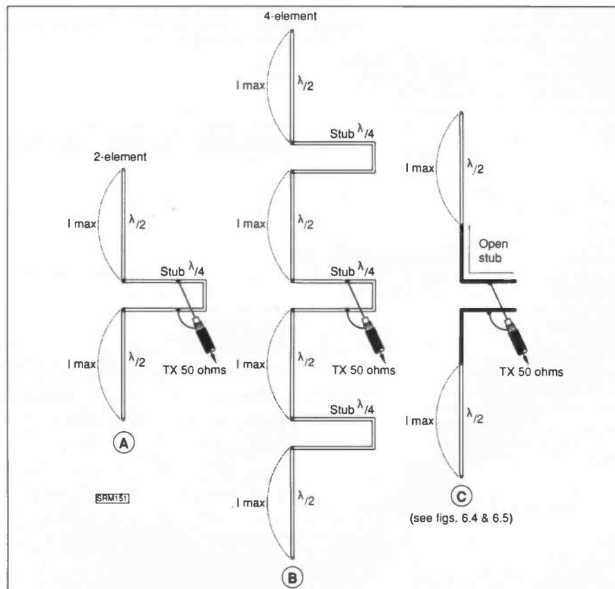
Fig. 6.3: Vertical collinear antenna configurations: (A) two close-spaced elements; (B) four close-spaced elements; (C) extended electrical spacing between two elements to obtain greater directivity gain.
