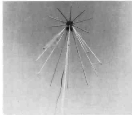
Fig. 6.1: Experimental discone omni-
