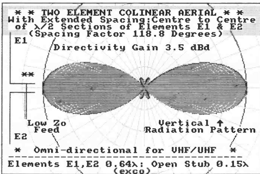
Fig. 6.4: Vertical radiation pattern of 2-element collinear with extended electrical spacing between centres of half-wave sections ( $0.66\lambda$ ,  $118.8^\circ$ ).
