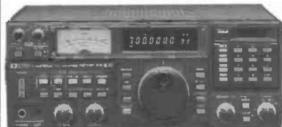
Listen in on public and private radio communications: weather, fire, coastguard TV, air-band and many, many more. Wideband frequency coverage provides you with all the channels you need to become a VHF and UHF listener. Turn on the infra-red remote control (optional) for 'armchair copy'. Frequency coverage is guaranteed to 1300MHz, starting at 25MHz, but may extend on individual units to 2GHz! Features include:
