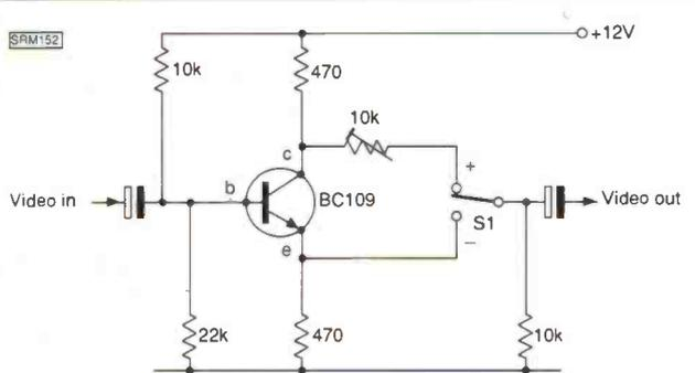
Fig. 3: External video inversion using a video modulator to allow the inverted signals to be viewed on a normal receiver. (Note that such a system does NOT convert SECAM to PAL).
