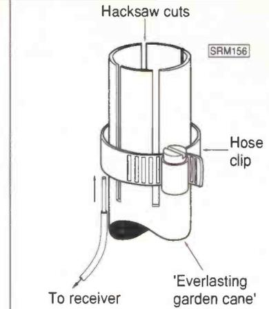
Fig. 1: Alternative jointing method
