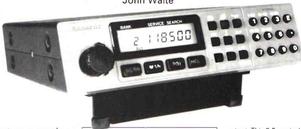
The BC-950XLT features coverage from 29MHz through to 956MHz in four bands though this is not continuous. The modern styling combined with its very compact size means that it will look good either in the car or shack.
