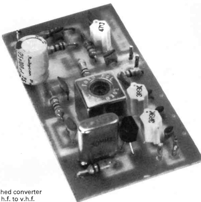
Finished converter with h.f. to v.h.f. option fitted.
