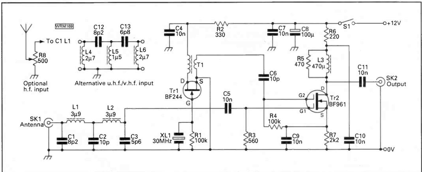
Fig. 1: Circuit diagram of h.f. to v.h.f. converter showing v.h.f. to v.h.f. options.
