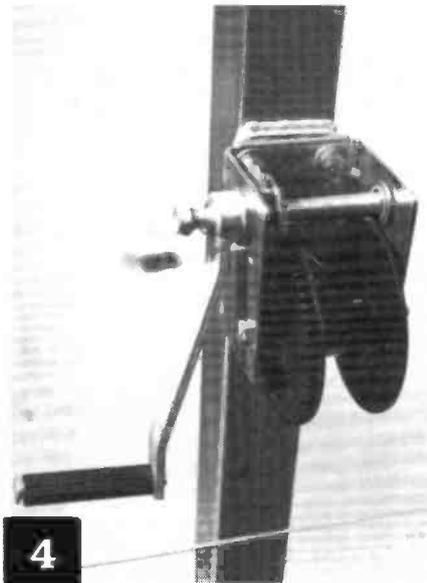
**4** This is the DL800 Friction Braked Winch, which Tennamast recommend. It provides easier and safer control of the mast during raising and lowering. The winch is bolted onto the ground post, as shown here, using the three bolts and washers provided. The positions of the three holes means that you cannot get it upside down. The handle is wound onto the shaft and the spring and Nyloc nut fitted and tightened to retain it.
