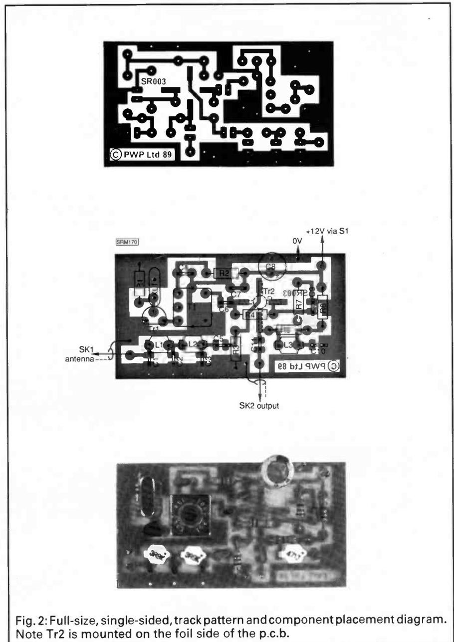
Fig. 2: Full-size, single-sided, track pattern and component placement diagram. Note Tr2 is mounted on the foil side of the p.c.b.
